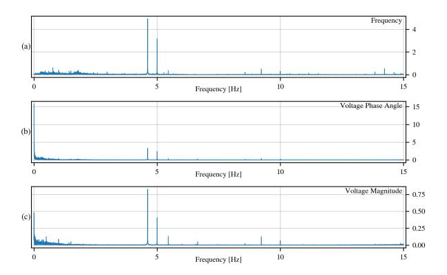
Figure 4.8: Absolute value of the Fourier transform over the positive frequency domain (0 to 15 Hz) of (a) frequency, (b) voltage phase angle, and (c) voltage magnitude of PMU k = 156 over quiet period #10 (see Table 4.1). Mean have been subtracted from the raw signal —to prevent a high peaks at frequency 0.
