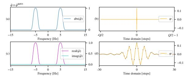
Figure 4.32: (a) Absolute value and (c) real and imaginary parts of filter vector  $\tilde{\varphi}^{\text{BPF5}}$  (M = 30); (b) and (d) show the component-wise absolute value of the inverse Fourier transform of  $\tilde{\varphi}^{\text{BPF5}}$ .
