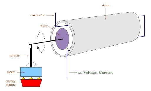
Figure 2.2: Turbine-Generator Model. A turbine converts different type of energy —such as steam or burnt natural gas— into rotation. The turbine shaft is connected to a generator shaft. A generator typically consists in a rotor (rotating part) that spins at a frequency  $\omega(t)$  inside a stator (static part). The rotation of the rotor creates a magnetic field that induces current into the conductor at frequency  $\omega(t)$ .
