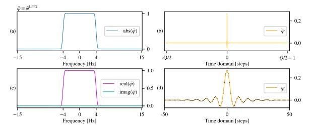
Figure 4.16: (a) Absolute value, (c) real and imaginary parts of filter vector  $\tilde{\varphi}^{\text{LPF4}}$  (M = 50); (b) and (d) show the component-wise absolute value of the inverse Fourier transform of  $\tilde{\varphi}^{\text{LPF4}}$ .
