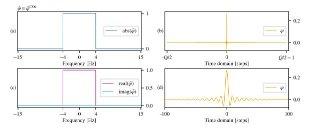
Figure 4.10: (a) Absolute value and (c) real and imaginary parts of filter vector  $\tilde{\varphi}^{\text{CO4}}$ ; (b) and (d) show the component-wise absolute value of the inverse Fourier transform of  $\tilde{\varphi}^{\text{CO4}}$ .
