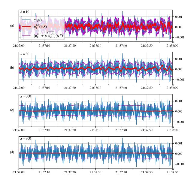
Figure 4.5: Frequency measurements with respect to a reference bus (in blue) of PMU k = 156 during one minute, between 9:37 and 9:38 PM on July 30, 2013. Average over sliding time horizon (in red) and a band of one standard deviation (in purple) are also shown for (a) S = 10, (b) S = 30, (c) S = 300, and (d) S = 900; corresponding to the number of samples made over 1/3, 1, 10, and 30 seconds, respectively.
