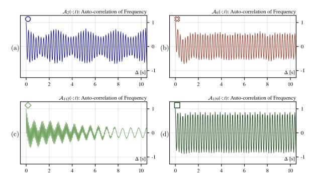
Figure 4.42: Auto-correlation functions for frequency for PMU's (a) k = 2, (b) k = 6, (c) k = 112, and (d) k = 139; at t=21:29:00 on July 30, 2013. The correlation matrices are constructed with the normalized time series  $\hat{m}^{(s)}(\cdot; S)$ , S = 30, T = 5400.
