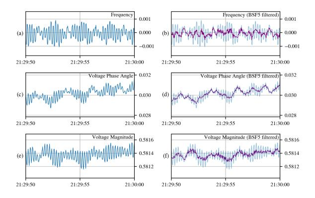
Figure 4.35: Original sampling (in blue) for (a) frequency, (c) voltage phase angle, and (e) voltage magnitude across 10 seconds on period #10 (see Table 4.1). Corresponding filtered series are shown (in purple) in plots (b), (d), and (f) using filtering vector  $\tilde{\varphi}^{\text{BSF5}}$ .
