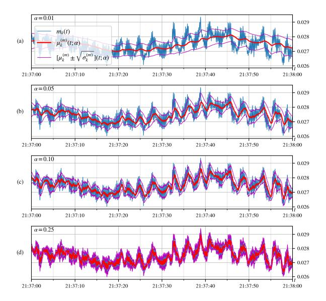
Figure 4.3: Voltage phase angle measurements with respect to a reference bus (in blue) of PMU k = 156 during one minute, between 9:37 and 9:38 PM on July 30, 2013. Moving average (in red) and a band of one standard deviation (in purple) are also shown for (a)  $\alpha = 0.01$ , (b)  $\alpha = 0.05$ , (c)  $\alpha = 0.10$ , and (d)  $\alpha = 0.25$ .
