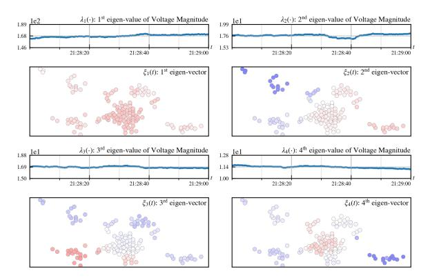
Figure 4.41: Largest four eigen-values from Figure 4.40 across the last minute before t, together with their corresponding normalized eigen-vectors at time t (positive values are shown in red, negative values are shown in blue). [t=21:29:00 on July 30, 2013]
