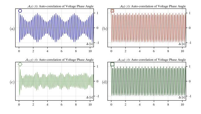
Figure A.3: Auto-correlation functions for voltage phase angle for PMU's (a) k = 2, (b) k = 6, (c) k = 112, and (d) k = 139; at t=21:29:00 on July 30, 2013. The correlation matrices are constructed with the normalized time series  $\hat{f}^{(s)}[\tilde{\varphi}^{\text{BPF5}}](\cdot; S)$  that has been filtered by a band-pass Fourier filter, S = 30, T = 5400.
