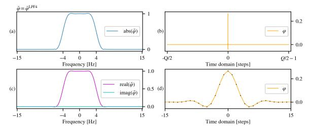
Figure 4.24: (a) Absolute value and (c) real and imaginary parts of filter vector  $\tilde{\varphi}^{\text{LPF4}}$  (M = 15); (b) and (d) show the component-wise absolute value of the inverse Fourier transform of  $\tilde{\varphi}^{\text{LPF4}}$ .
