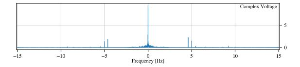
Figure 4.9: Absolute value of the Fourier transform of the complex voltage of PMU k = 156 over quiet period #10. Again, mean have been subtracted from the raw signal.
