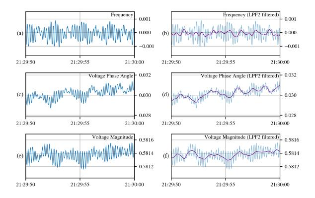
Figure 4.21: Original sampling (in blue) for (a) frequency, (c) voltage phase angle, and (e) voltage magnitude across 10 seconds on period #10 (see Table 4.1). Corresponding filtered series are shown (in purple) in plots (b), (d), and (f) using filtering vector  $\tilde{\varphi}^{\text{LPF2}}$ .
