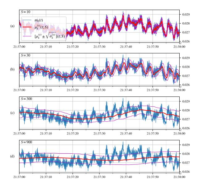
Figure 4.6: Voltage phase angle measurements with respect to a reference bus (in blue) of PMU k = 156 during one minute, between 9:37 and 9:38 PM on July 30, 2013. Average over sliding time horizon (in red) and a band of one standard deviation (in purple) are also shown for (a) S = 10, (b) S = 30, (c) S = 300, and (d) S = 900; corresponding to the number of samples made over 1/3, 1, 10, and 30 seconds, respectively.
