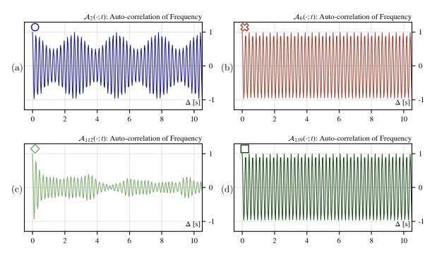
Figure 4.44: Auto-correlation functions for frequency for PMU's (a) k = 2, (b) k = 6, (c) k = 112, and (d) k = 139; at t=21:29:00 on July 30, 2013. The correlation matrices are constructed with the normalized time series  $\hat{f}^{(s)}[\tilde{\varphi}^{\text{BPF5}}](\cdot; S)$ , S = 30, T = 5400.
