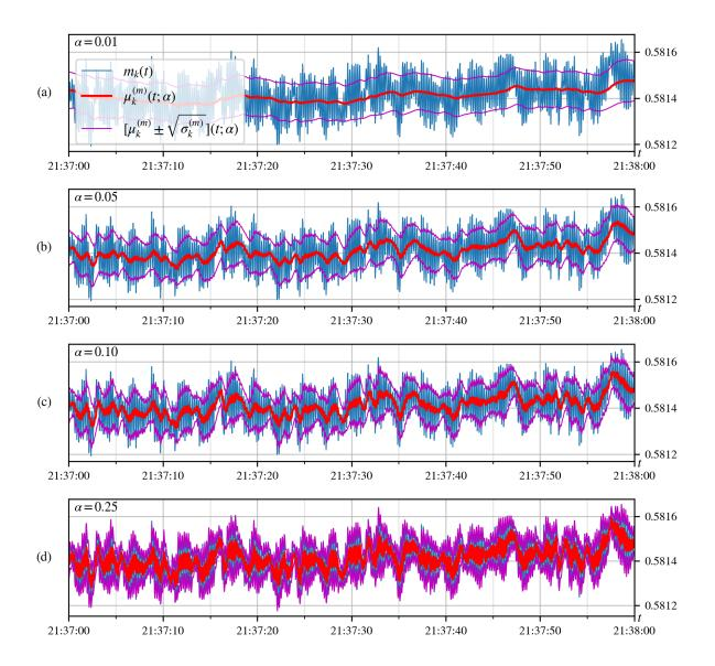
Figure 4.4: Voltage magnitude measurements with respect to bus nominal value (in blue) of PMU k = 156 during one minute, between 9:37 and 9:38 PM on July 30, 2013. Moving average (in red) and a band of one standard deviation (in purple) are also shown for (a)  $\alpha = 0.01$ , (b)  $\alpha = 0.05$ , (c)  $\alpha = 0.10$ , and (d)  $\alpha = 0.25$ .
