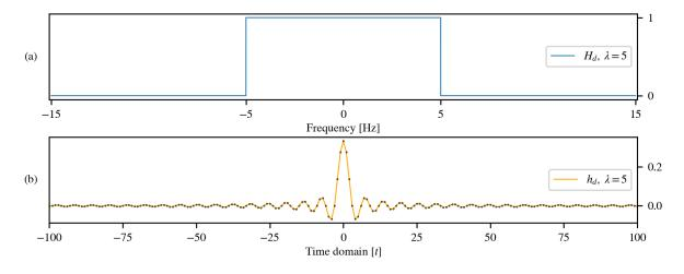
Figure 4.14: (a) Desired frequency response  $H_d$  for cut-off frequency  $\lambda = 5$  Hz and (b) its infinite impulse response (showing for t between -100 and 100).
