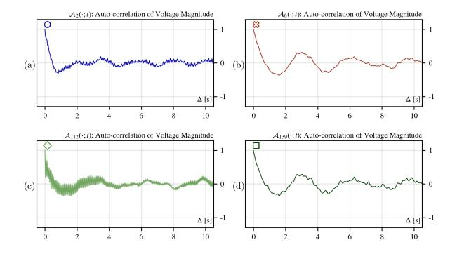
Figure A.6: Auto-correlation functions for voltage magnitude for PMU's (a) k = 2, (b) k = 6, (c) k = 112, and (d) k = 139; at t=21:29:00 on July 30, 2013. The correlation matrices are constructed with the normalized time series  $\hat{f}^{(s)}[\tilde{\varphi}^{\text{BSF5}}](\cdot; S)$  that has been filtered by a band-stop Fourier filter, S = 30, T = 5400.
