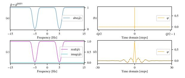
Figure 4.34: (a) Absolute value and (c) real and imaginary parts of filter vector  $\tilde{\varphi}^{\text{BSF5}}$  (M = 30); (b) and (d) show the component-wise absolute value of the inverse Fourier transform of  $\tilde{\varphi}^{\text{BSF5}}$ .
