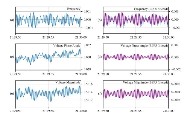
Figure 4.33: Original sampling (in blue) for (a) frequency, (c) voltage phase angle, and (e) voltage magnitude across 10 seconds on period #10 (see Table 4.1). Corresponding filtered series are shown (in purple) in plots (b), (d), and (f) using filtering vector  $\tilde{\varphi}^{\text{BPF5}}$ .
