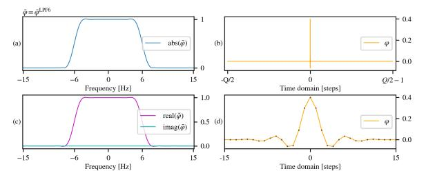
Figure 4.28: (a) Absolute value and (c) real and imaginary parts of filter vector  $\tilde{\varphi}^{\text{LPF6}}$  (M = 15); (b) and (d) show the component-wise absolute value of the inverse Fourier transform of  $\tilde{\varphi}^{\text{LPF6}}$ .
