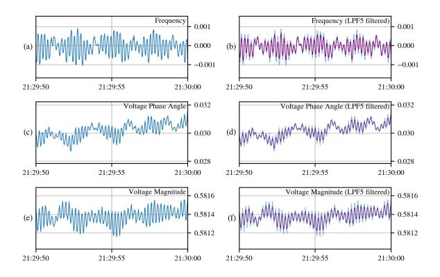
Figure 4.27: Original sampling (in blue) for (a) frequency, (c) voltage phase angle, and (e) voltage magnitude across 10 seconds on period #10 (see Table 4.1). Corresponding filtered series are shown (in purple) in plots (b), (d), and (f) using filtering vector  $\tilde{\varphi}^{\text{LPF5}}$ .
