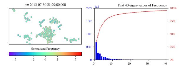
Figure 4.36: Left: normalized frequency  $\hat{m}^{(s)}(t; S)$  representing each PMU in its geographical location. Right: First 40 eigen-values of  $\Sigma_0(t; T; \hat{m}^{(s)}(\cdot; S))$  in blue, and its spectral contribution in red. [t=21:29:00 on July 30, 2013; S = 30; T = 5400]
