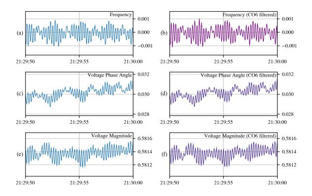
Figure 4.13: Original sampling (in blue) for (a) frequency, (c) voltage phase angle, and (e) voltage magnitude across 10 seconds on period #10 (see Table 4.1). Corresponding filtered series are shown (in purple) in plots (b), (d), and (f) using filtering vector  $\tilde{\varphi}^{CO6}$ .
