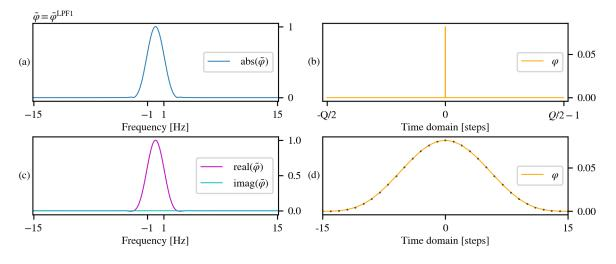
Figure 4.18: (a) Absolute value and (c) real and imaginary parts of filter vector  $\tilde{\varphi}^{\text{LPF1}}$  (M = 15); (b) and (d) show the component-wise absolute value of the inverse Fourier transform of  $\tilde{\varphi}^{\text{LPF1}}$ .
