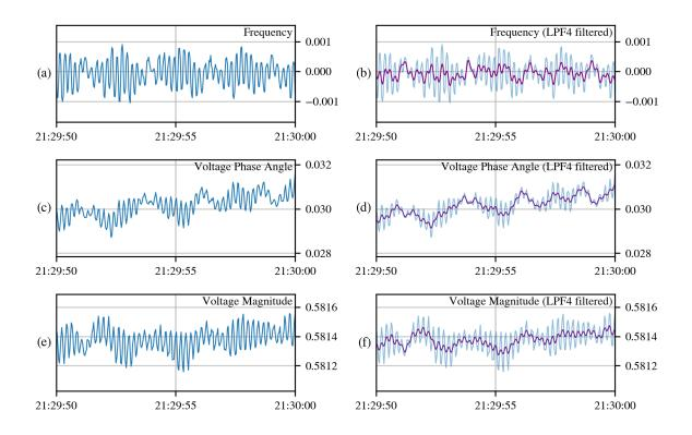
Figure 4.25: Original sampling (in blue) for (a) frequency, (c) voltage phase angle, and (e) voltage magnitude across 10 seconds on period #10 (see Table 4.1). Corresponding filtered series are shown (in purple) in plots (b), (d), and (f) using filtering vector  $\tilde{\varphi}^{\text{LPF4}}$ .
