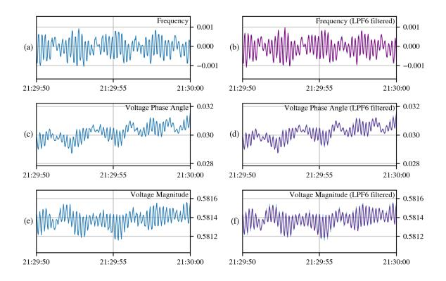
Figure 4.29: Original sampling (in blue) for (a) frequency, (c) voltage phase angle, and (e) voltage magnitude across 10 seconds on period #10 (see Table 4.1). Corresponding filtered series are shown (in purple) in plots (b), (d), and (f) using filtering vector  $\tilde{\varphi}^{\text{LPF6}}$ .
