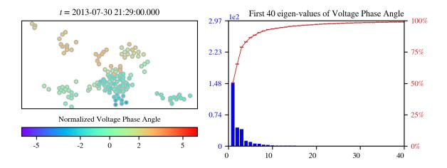
Figure 4.38: Left: normalized voltage phase angle  $\hat{m}^{(s)}(t; S)$  representing each PMU in its geographical location. Right: First 40 eigen-values of  $\Sigma_0(t; T; \hat{m}^{(s)}(\cdot; S))$  in blue, and its spectral contribution in red. [t=21:29:00 on July 30, 2013; S = 30; T = 5400]
