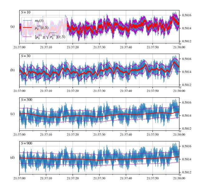
Figure 4.7: Voltage magnitude measurements with respect to bus nominal value (in blue) of PMU k = 156 during one minute, between 9:37 and 9:38 PM on July 30, 2013. Average over sliding time horizon (in red) and a band of one standard deviation (in purple) are also shown for (a) S = 10, (b) S = 30, (c) S = 300, and (d) S = 900; corresponding to the number of samples made over 1/3, 1, 10, and 30 seconds, respectively.
