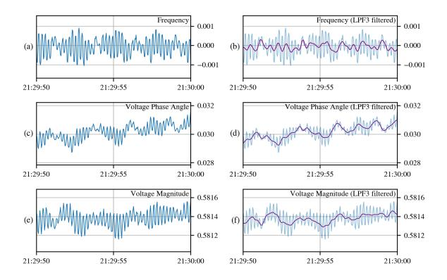
Figure 4.23: Original sampling (in blue) for (a) frequency, (c) voltage phase angle, and (e) voltage magnitude across 10 seconds on period #10 (see Table 4.1). Corresponding filtered series are shown (in purple) in plots (b), (d), and (f) using filtering vector  $\tilde{\varphi}^{\text{LPF3}}$ .
