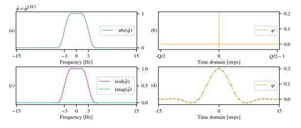
Figure 4.22: (a) Absolute value and (c) real and imaginary parts of filter vector  $\tilde{\varphi}^{\text{LPF3}}$  (M = 15); (b) and (d) show the component-wise absolute value of the inverse Fourier transform of  $\tilde{\varphi}^{\text{LPF3}}$ .
