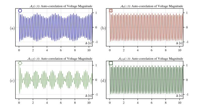
Figure A.7: Auto-correlation functions for voltage magnitude for PMU's (a) k = 2, (b) k = 6, (c) k = 112, and (d) k = 139; at t=21:29:00 on July 30, 2013. The correlation matrices are constructed with the normalized time series  $\hat{f}^{(s)}[\tilde{\varphi}^{\text{BPF5}}](\cdot; S)$  that has been filtered by a band-pass Fourier filter, S = 30, T = 5400.
