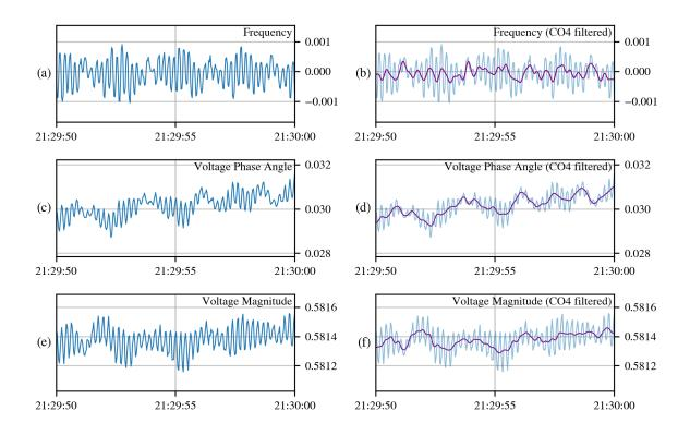
Figure 4.11: Original sampling (in blue) for (a) frequency, (c) voltage phase angle, and (e) voltage magnitude across 10 seconds on period #10 (see Table 4.1). Corresponding filtered series are shown (in purple) in plots (b), (d), and (f) using filtering vector  $\tilde{\varphi}^{CO4}$ .
