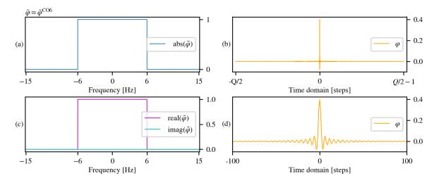
Figure 4.12: (a) Absolute value and (c) real and imaginary parts of filter vector  $\tilde{\varphi}^{CO6}$ ; (b) and (d) show the component-wise absolute value of the inverse Fourier transform of  $\tilde{\varphi}^{CO6}$ .
