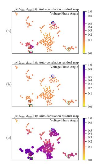
Figure A.4: Residue of auto-correlation functions for voltage phase angle using (a)  $\hat{m}^{(s)}(\cdot; S)$ , (b)  $\hat{f}^{(s)}[\tilde{\varphi}^{\text{BSF5}}](\cdot; S)$ , and (c)  $\hat{f}^{(s)}[\tilde{\varphi}^{\text{BPF5}}](\cdot; S)$ ; at t=21:29:00 on July 30, 2013, with S=30, T=5400,  $\Delta_{\min}=30$ , and  $\Delta_{\max}=1800$ . Geometrical figures show the position of the sensors depicted in Figures A.1–A.3.
