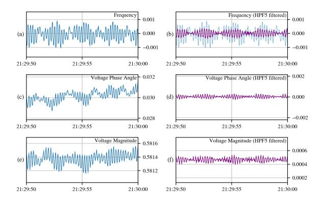
Figure 4.31: Original sampling (in blue) for (a) frequency, (c) voltage phase angle, and (e) voltage magnitude across 10 seconds on period #10 (see Table 4.1). Corresponding filtered series are shown (in purple) in plots (b), (d), and (f) using filtering vector  $\tilde{\varphi}^{\text{HPF5}}$ .
