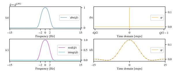
Figure 4.20: (a) Absolute value and (c) real and imaginary parts of filter vector  $\tilde{\varphi}^{\text{LPF2}}$  (M = 15); (b) and (d) show the component-wise absolute value of the inverse Fourier transform of  $\tilde{\varphi}^{\text{LPF2}}$ .
