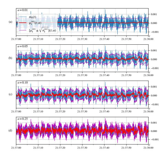
Figure 4.2: Frequency measurements with respect to a reference bus (in blue) of PMU k = 156 during one minute, between 9:37 and 9:38 PM on July 30, 2013. Moving average (in red) and a band of one standard deviation (in purple) are also shown for (a)  $\alpha = 0.01$ , (b)  $\alpha = 0.05$ , (c)  $\alpha = 0.10$ , and (d)  $\alpha = 0.25$ .
