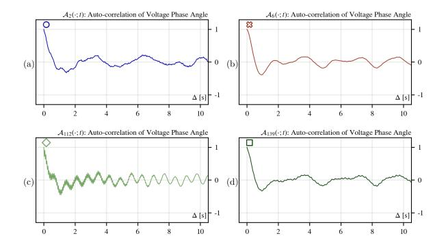
Figure A.2: Auto-correlation functions for voltage phase angle for PMU's (a) k = 2, (b) k = 6, (c) k = 112, and (d) k = 139; at t=21:29:00 on July 30, 2013. The correlation matrices are constructed with the normalized time series  $\hat{f}^{(s)}[\tilde{\varphi}^{\text{BSF5}}](\cdot; S)$  that has been filtered by a band-stop Fourier filter, S = 30, T = 5400.
