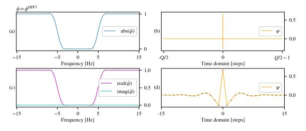
Figure 4.30: (a) Absolute value and (c) real and imaginary parts of filter vector  $\tilde{\varphi}^{\text{HPF5}}$  (M = 15); (b) and (d) show the component-wise absolute value of the inverse Fourier transform of  $\tilde{\varphi}^{\text{HPF5}}$ .
