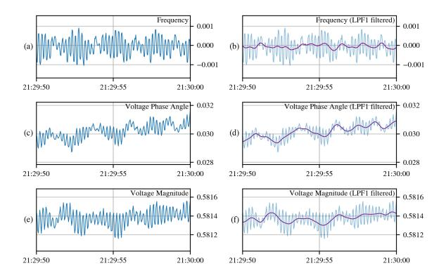
Figure 4.19: Original sampling (in blue) for (a) frequency, (c) voltage phase angle, and (e) voltage magnitude across 10 seconds on period #10 (see Table 4.1). Corresponding filtered series are shown (in purple) in plots (b), (d), and (f) using filtering vector  $\tilde{\varphi}^{\text{LPF1}}$ .
