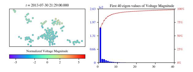
Figure 4.40: Left: normalized voltage magnitude  $\hat{m}^{(s)}(t; S)$  representing each PMU in its geographical location. Right: First 40 eigen-values of  $\Sigma_0(t; T; \hat{m}^{(s)}(\cdot; S))$  in blue, and its spectral contribution in red. [t=21:29:00 on July 30, 2013; S = 30; T = 5400]
