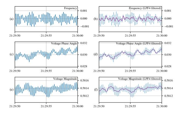
Figure 4.17: Original sampling (in blue) for (a) frequency, (c) voltage phase angle, and (e) voltage magnitude across 10 seconds on period #10 (see Table 4.1). Corresponding filtered series are shown (in purple) in plots (b), (d), and (f) using filtering vector  $\tilde{\varphi}^{\text{LPF4}}$ .
