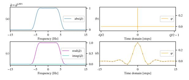
Figure 4.26: (a) Absolute value and (c) real and imaginary parts of filter vector  $\tilde{\varphi}^{\text{LPF5}}$  (M = 15); (b) and (d) show the component-wise absolute value of the inverse Fourier transform of  $\tilde{\varphi}^{\text{LPF5}}$ .
