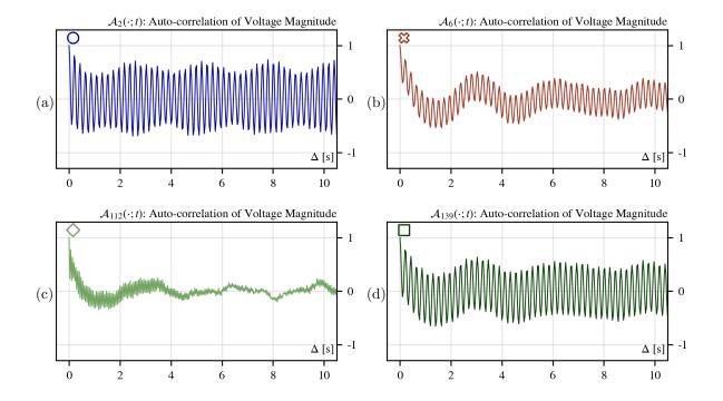
Figure A.5: Auto-correlation functions for voltage magnitude for PMU's (a) k = 2, (b) k = 6, (c) k = 112, and (d) k = 139; at t=21:29:00 on July 30, 2013. The correlation matrices are constructed with the normalized time series  $\hat{m}^{(s)}(\cdot; S)$ , S = 30, T = 5400.
