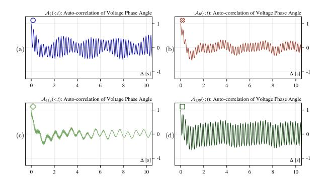
Figure A.1: Auto-correlation functions for voltage phase angle for PMU's (a) k = 2, (b) k = 6, (c) k = 112, and (d) k = 139; at t=21:29:00 on July 30, 2013. The correlation matrices are constructed with the normalized time series  $\hat{m}^{(s)}(\cdot; S)$ , S = 30, T = 5400.
