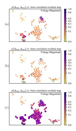
Figure A.8: Residue of auto-correlation functions for voltage magnitude using (a)  $\hat{m}^{(s)}(\cdot; S)$ , (b)  $\hat{f}^{(s)}[\tilde{\varphi}^{\text{BSF5}}](\cdot; S)$ , and (c)  $\hat{f}^{(s)}[\tilde{\varphi}^{\text{BPF5}}](\cdot; S)$ ; at t=21:29:00 on July 30, 2013, with S=30, T=5400,  $\Delta_{\min}=30$ , and  $\Delta_{\max}=1800$ . Geometrical figures show the position of the sensors depicted in Figures A.5–A.7.
