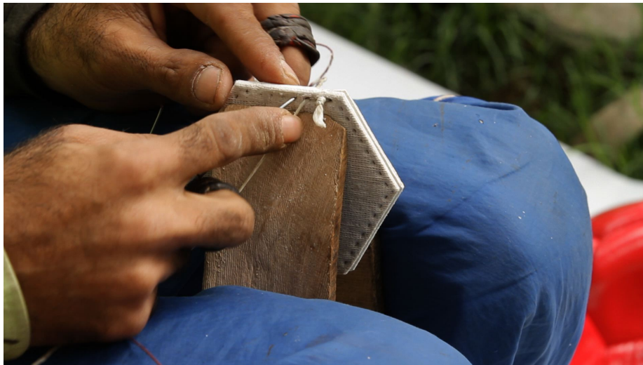
Figure A.6: Stitching (Step 4)
