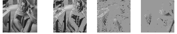
Fig. 5. The segmentation of the 4,096 image blocks from the Barbara image. The image (left) is segmented into three groups (right three). Roughly speaking, the first subspace contains mostly image blocks with homogeneous textures; the second and third subspaces contain blocks with textures of different spatial orientations and frequencies.
