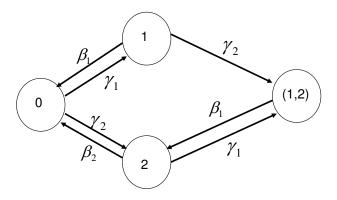
$\gamma_j$  = rate copier *j* fails,  $\beta_j$  = rate copier *j* repaired
