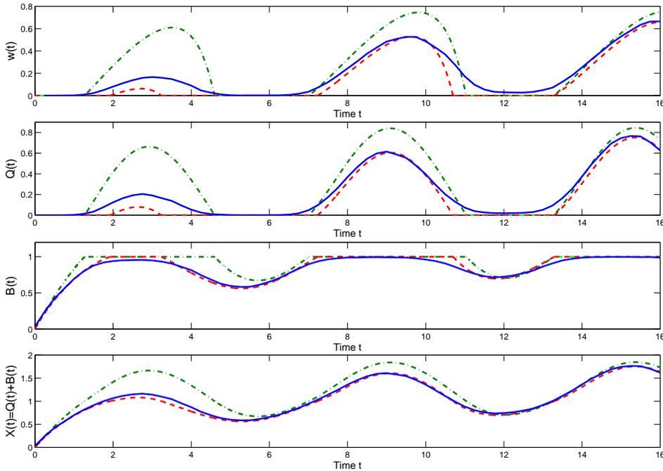
**Fig. 3** Simulation comparison for the  $M_t/H_2/s + E_2$  fluid model: (i) the averages of 200 sample paths of the scaled queueing model based on  $n = 30$  (blue solid lines), (ii) fluid functions (red dashed lines) and (iii) fluid functions assuming  $M$  service (green dashed lines).
