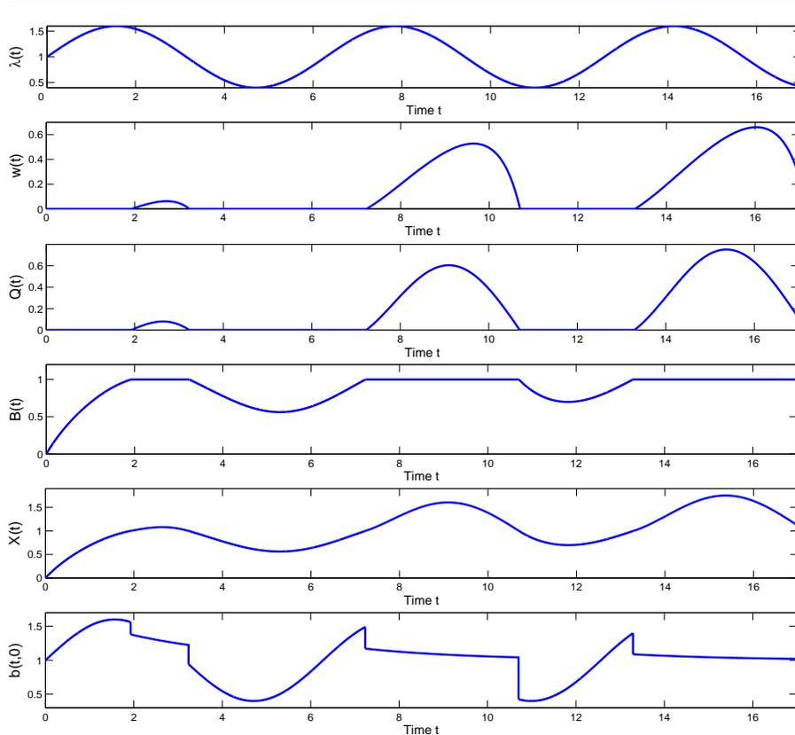
**Fig. 1** The performance functions of the  $G_t/H_2/s + E_2$  fluid model with sinusoidal arrival-rate function: (i) arrival rate  $\lambda(t)$ ; (ii) head-of-line waiting time  $w(t)$ ; (iii) fluid waiting in queue  $Q(t)$ ; (iv) fluid in service  $B(t)$ ; (v) total fluid in system  $X(t)$ ; (vi) rate into service  $b(t,0)$ .
