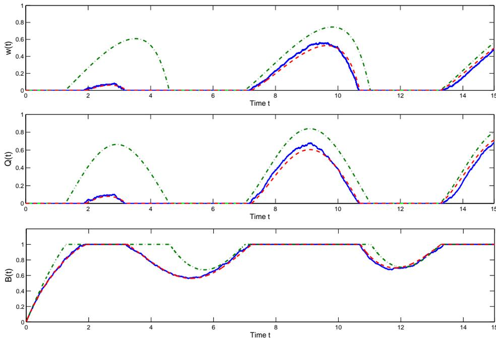
**Fig. 2** Simulation comparison for the  $M_t/H_2/s + E_2$  fluid model: (i) single sample paths in the scaled queueing model based on  $n = 2000$  (blue solid lines), (ii) fluid functions (red dashed lines) and (iii) fluid functions assuming  $M$  service (green dashed lines).
