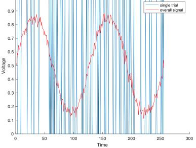
The averaged result using a 1 bit converter is surprisingly similar to the signal average in the previous example. This shows us how reasonable averaging results can be obtained with a low-resolution ADC using the statistical properties of the noise component. This suggests that the ADC resolution may not be a critical component in the signal averaging technique.
