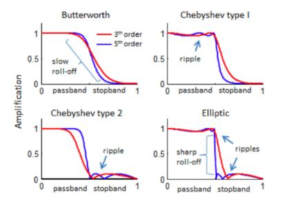
An important parameter when setting up a filter is the *filter order*. The order refers to the number of coefficients used in determining the filter function. It will determine the balance between time versus. frequency resolution.
