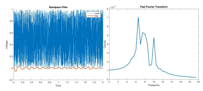
In this example, the amplitude of each frequency between 6 to 10 Hz is quite variable. This is a result of the short time period of our sample and the chance outcome of our random number generator. The non-zero values before 6 Hz and after 10 Hz demonstrate one tradeoff in using the Butterworth filter: there will be a relatively smooth roll-off in the stopband, with the advantage that we don't introduce ripples.
