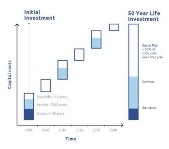
The renovation and modernization of the services and space plan of a building contribute far more to its lifecycle costs than the structure. Changes to the space plan alone comprise more than 50% of the total capital costs over the lifetime of a building. Diagram by C-Lab, based on a diagram by Frank Duffy in *Work and the City* (London: Black Dog, 2008).
