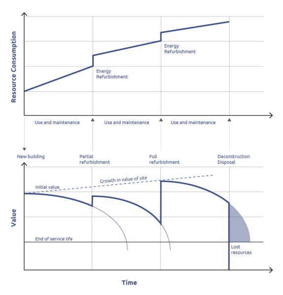
Life cycle assessments take into account the service life and replacement cost of building components, as well as the embodied and operating energy used over each period. Diagram by C-Lab, based on diagram from Holger Konig, et al. *A Life Cycle Approach To Buildings. Principles, Calculations, Tools.* Munich: Edition Detail Books, 2010.
