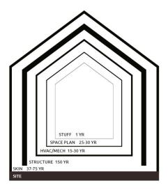
A building is comprised of many layers, each with different timescales for renovation and replacement.
