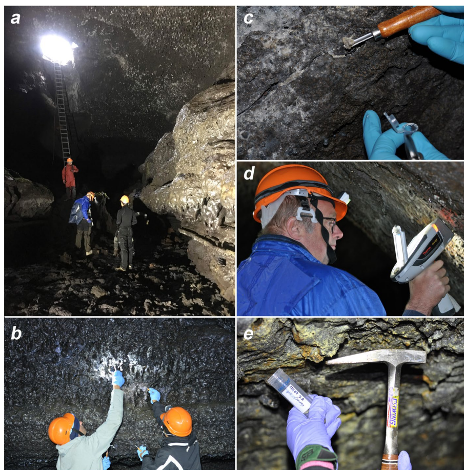
Figure 3. Sampling strategy. (a) Cave entrance to cave H, 12 m below ground. (b) Sampling in pairs: one sampler and one assistant handling cleaning and handing over of tools. (c) Biological sampling (step 2): scraping mats from the cave wall. (d) Handheld X-ray fluorescence measurements of cave wall (step 4). (e) Substrate sampling with a geological hammer and Falcon tube (steps 3 and 5).
