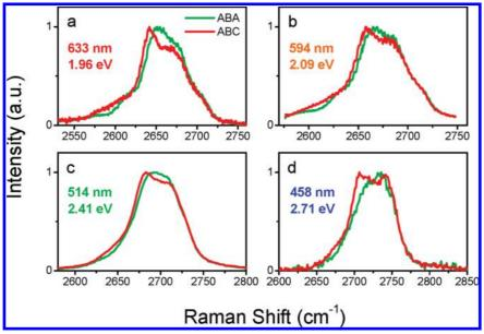
FIGURE 2. Raman spectra of the 2D-mode of ABA (green line) and ABC (red line) trilayer graphene samples at four different laser excitation wavelengths. The increase in the average Raman shift with excitation photon energy is an expected consequence of the double-resonance process that selectively couples phonons with different momenta around the K-point.
