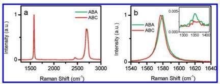
FIGURE 3. Raman spectra of graphene trilayers with ABA (green line) and ABC (red line) stacking order. (a) Raman spectra over a broad energy range. (b) Details of G-mode and D-mode (inset) spectra. The excitation laser wavelength is 514 nm.
