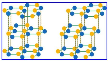
FIGURE 1. Lattice structure of trilayer graphene with ABA (left) and ABC (right) stacking sequence. The yellow and blue dots represent carbon atoms in the A and B sublattices of the graphene honeycomb structure.
