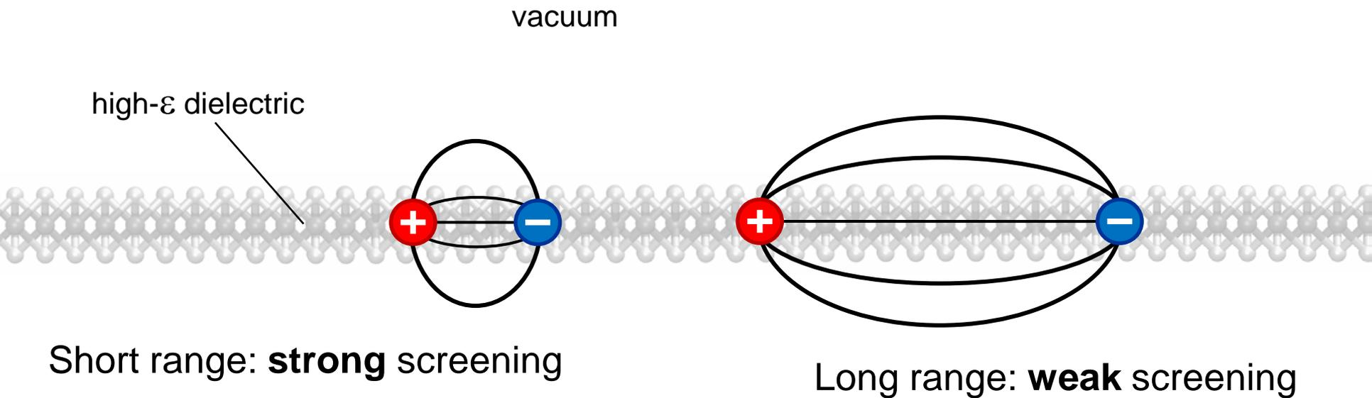
Electric field fringes out of 2D graphene into vacuum
