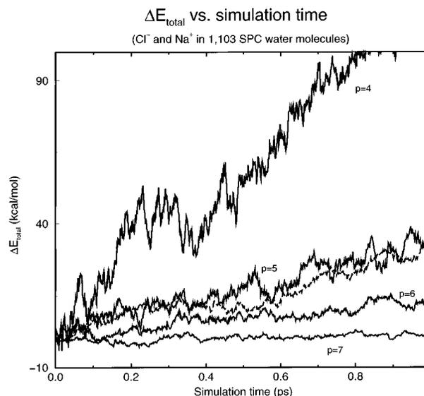
FIG. 1. Energy conservation for different force algorithms, using the Verlet integrator. The system studied contained one  $\text{Cl}^-$  and one  $\text{Na}^+$  ion, plus 1103 SPC water molecules. The dashed line corresponds to a simulation using the Ewald summation method ( $r_c = 9 \text{ \AA}$ ,  $\eta = 5.5$ ,  $k_{\text{max}} = 5$ ); the others are for simulations using the FMM with different number of multipoles ( $p$ ).
