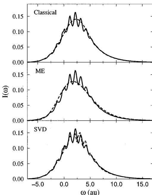
FIG. 2. The electronic absorption spectrum of the chromophore coupled to optical phonons. The solid line in all three panels is the fully quantum result. The dashed lines from top to bottom are as follows: (1) the classical Franck–Condon spectrum; (2) the spectrum reconstructed by the maximum entropy method; (3) the spectrum reconstructed by the singular value decomposition method.
