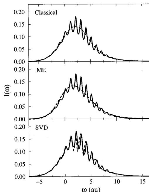
FIG. 1. The electronic absorption spectrum of the chromophore coupled to acoustic phonons. The solid line in all three panels is the fully quantum result. The dashed lines from top to bottom are as follows: (1) the classical Franck–Condon spectrum; (2) the spectrum reconstructed by the maximum entropy method; (3) the spectrum reconstructed by the singular value decomposition method.
