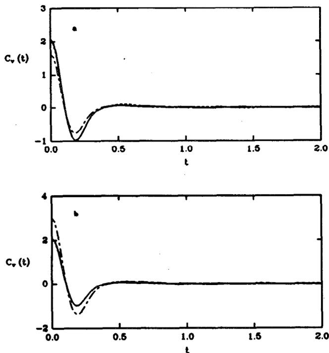
FIG. 1. (a) The unnormalized velocity correlation functions defined in Eq. (3.1) as a function of time for the light particles in the Lennard-Jones mixture for the light particles for RESPA (solid line), velocity Verlet (dashed line), and for TJMTS (dash-dot line). (b) The same as (a), but using a different initial configuration.
