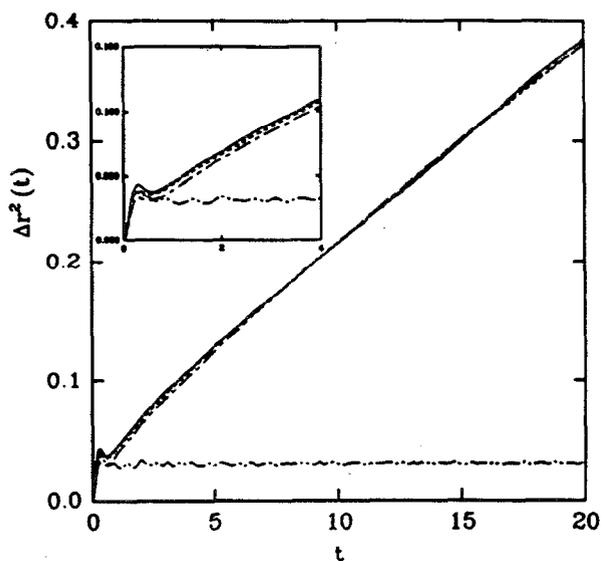
FIG. 2. The mean-square displacements defined in Eq. (3.2) as a function of time for the light particles in the Lennard-Jones mixture for the light particles for RESPA (solid line), velocity Verlet (dashed line), TJMTS (dash-dot line), and for motion of the light particles in a fixed heavy particle matrix with the same initial conditions as in Fig. 1(a) (dash-double dot line).
