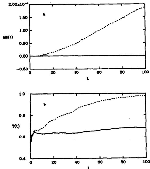
FIG. 4. (a) The instantaneous deviation in the energy from the initial value, normalized by the initial value for RESPA (solid line) and TJMTS (dashed line). (b) The cumulative average temperature of the light particles for RESPA (solid line) and TJMTS (dashed line).
