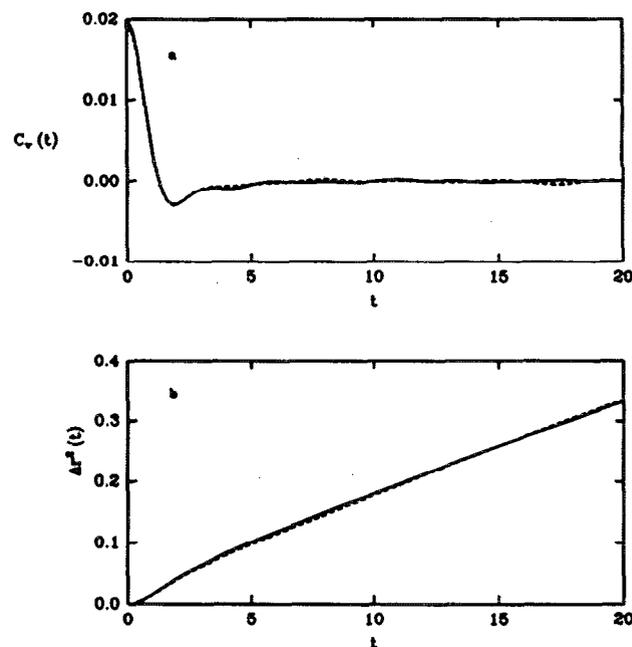
FIG. 3. (a) The velocity autocorrelation function for the heavy particles as computed by RESPA (solid line) and by TJMTS (dashed line). (b) The mean square displacement for the heavy particles as computed by RESPA (solid line) and TJMTS (dashed line).
