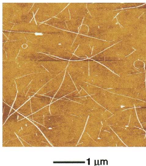
Figure 3. A typical AFM height image of SWNTs deposited on an -\text{NH}_2 functionalized glass coverslip. The z range is 10 nm.
