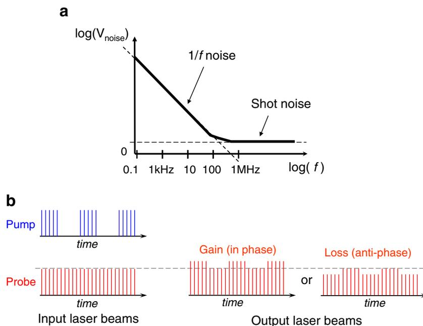
**Fig. 2** Principle of high-frequency modulation scheme. **a** Noise spectrum (log–log plot) of a typical laser source as a function of frequency  $f$ . In the low-frequency range (from DC to kilohertz), the noise follows the so-called  $1/f$  noise. In the higher-frequency range, the noise approaches the flat floor of shot noise. The high-frequency modulation scheme creates and subsequently detects the signal at a high frequency
