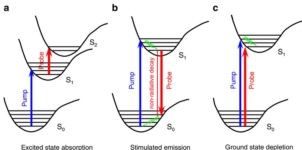
are extremely brief (less than 1 ps). Besides, the pump and probe pulse trains do not need to overlap in time. In fact, the probe pulse train is delayed by a few hundred femtoseconds with respect to the pump pulse train to permit the molecule enough time to relax vibrationally in the electronic excited state. This delay is also useful to separate the excited state absorption signal from other instantaneous nonlinear optical processes such as stimulated Raman scattering [13].
