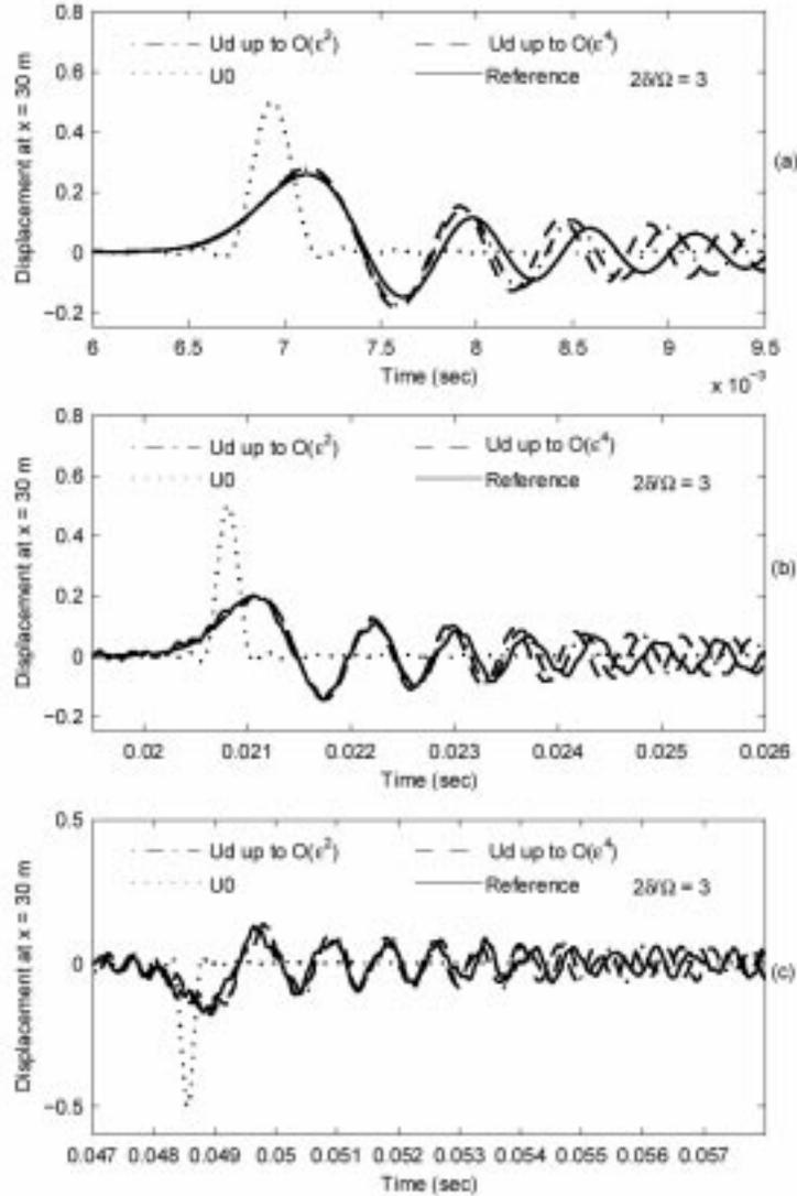
Figure 4: Displacements at  $x = 30m$  for the initial half pulse width  $\delta = 0.3m$
