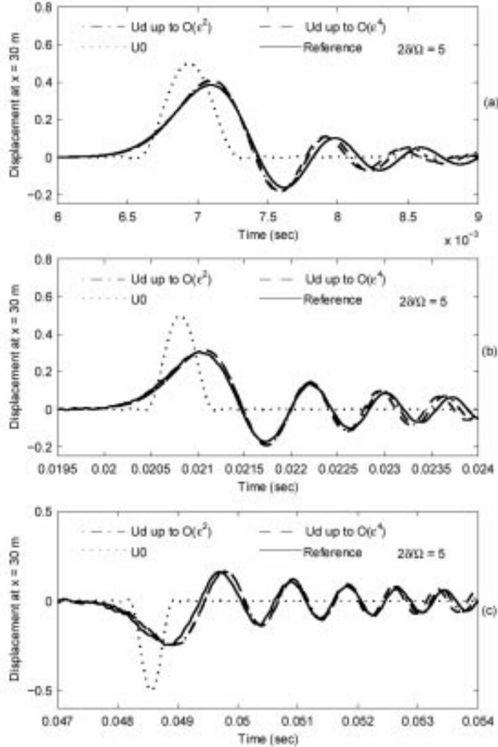
Figure 3: Displacements at  $x = 30m$  for the initial half pulse width  $\delta = 0.5m$
