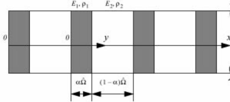
Figure 1: A bilaminate with a periodic microstructure
