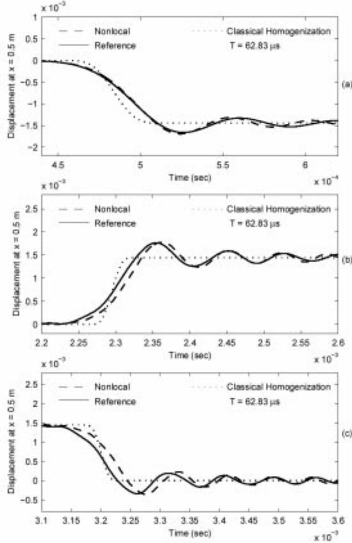
Figure 4: The response with an impact load (pulse duration  $T = 62.83\mu s$ ).
