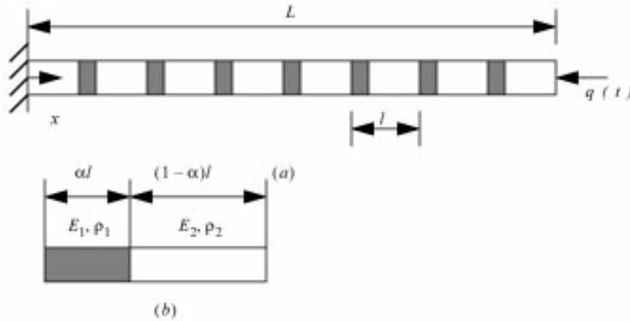
Figure 1: A bilaminate with periodic microstructure
