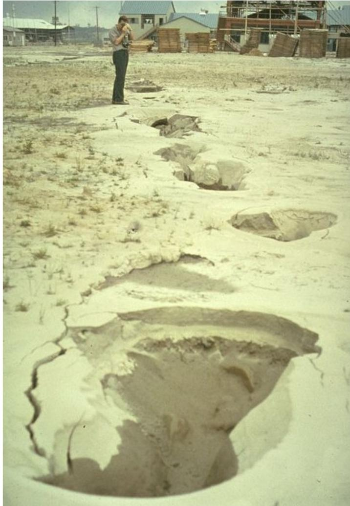
Fig. 4. Effects of sand boils due to liquefaction, Niigata, 1964. (Photo from National Information Service for Earthquake Engineering, University of California, Berkeley)
