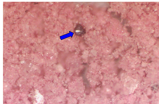
Figure 13: Optical microscope observation, 100x magnification: Dredge material from Port Newark dried at 500°C, note: agglomerate around oil product (arrow)
