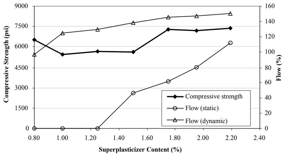
**Fig. 6.3: Summary - Flow (static) at w/c=0.47**
