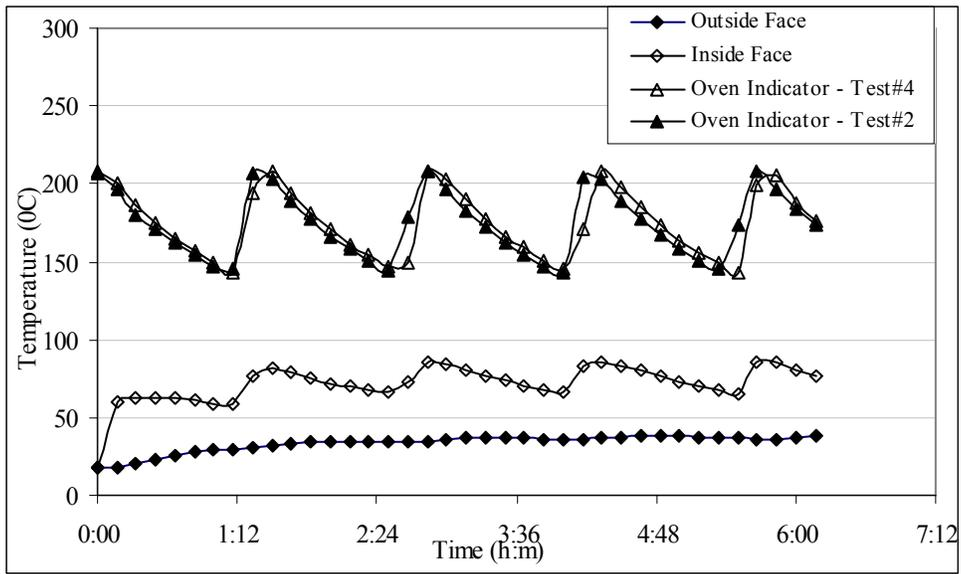
Fig. 9.6: Temperature Histories, Test #4 (Sample 77 - 10% fiber) – Procedure II
