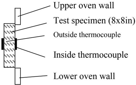
Fig. 9.1: Schematic diagram showing the thermocouple sensor positions.
