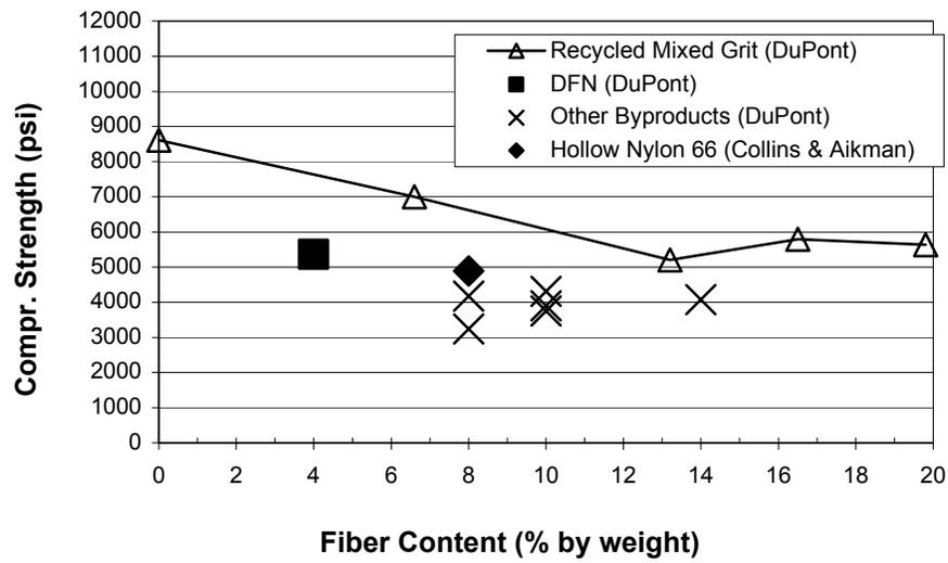
Fig. 16.1 Effect of fiber content on 7-day strength (Flow > 90, w/c = 0.34)
