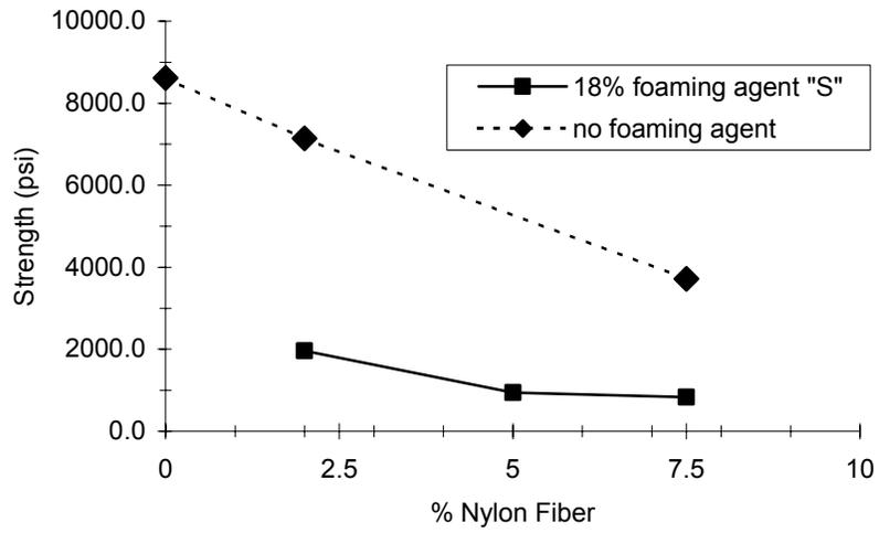
Fig. 11.1: Strength vs. amount of nylon fiber.
