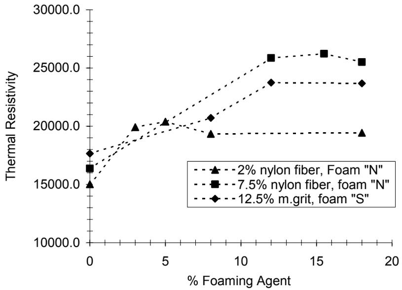
Fig. 11.5: Thermal resistivity vs. amount of foaming agent and type of fiber.
