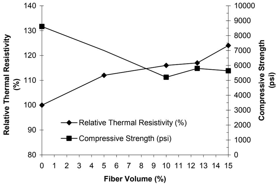
Fig. 10.1: Thermal Resistivity and Compressive Strength vs. Fiber Content – Recycled Grit (mixed Fiber)
