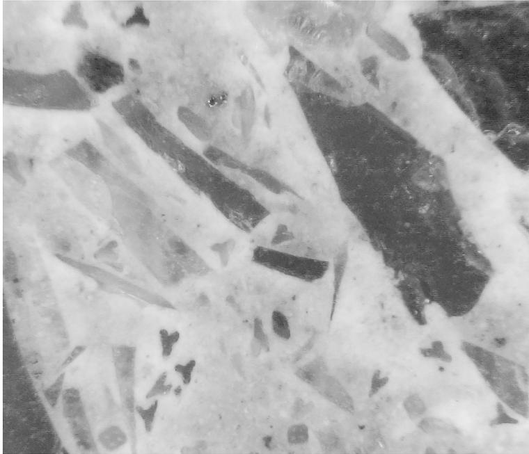
Fig. 18.6 Optical microscope image of glass concrete sample after 700 freeze-thaw cycles
