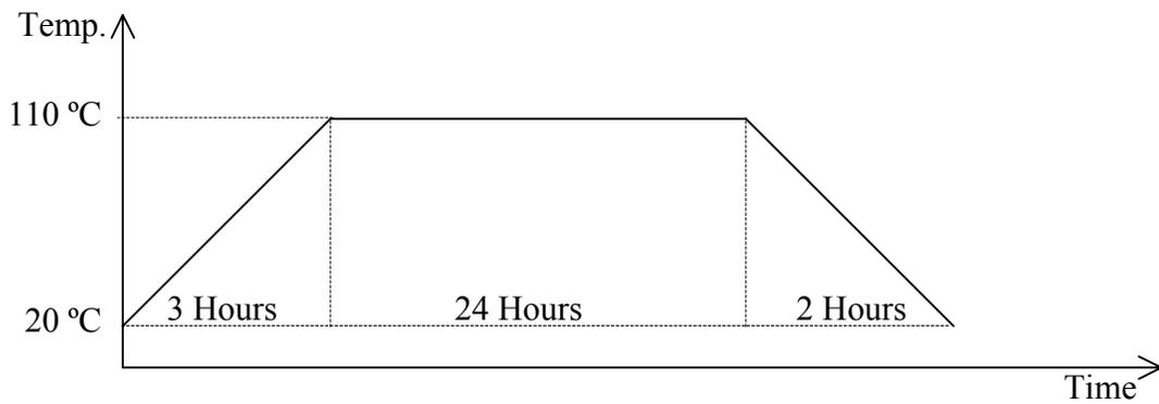
Fig. 9.2: Heating cycle for drying of specimens.
