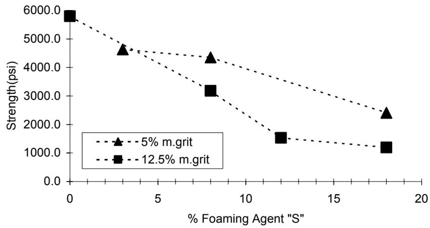
Fig. 11.2: Strength vs. amount of foaming agent "S".
