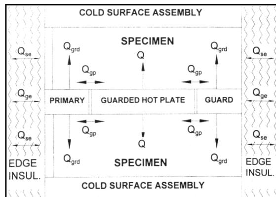
Fig 17.2 Illustration of Idealized Heat Flow in a Guarded-Hot-Plate Apparatus
