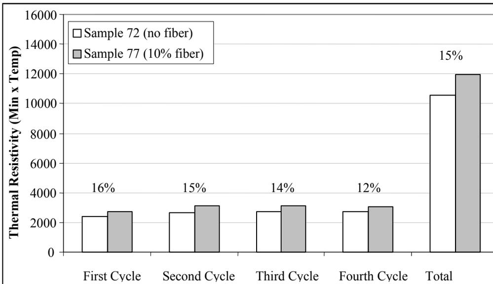
Fig. 9.9: Effect of Fiber on Thermal Resistivity (Procedure II - Test Period 6 hours)
