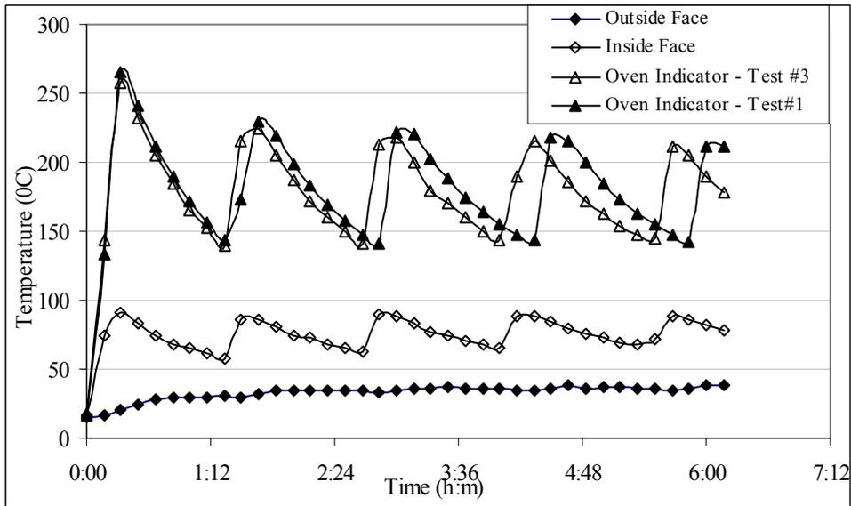
Fig. 9.5: Temperature Histories, Test #3 (Sample 77 - 10% fiber) – Procedure I
