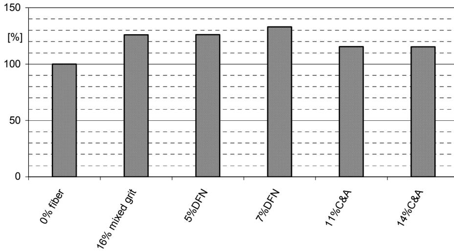
Fig. 16.4 Thermal performance of mixes with various recycled fibers.
