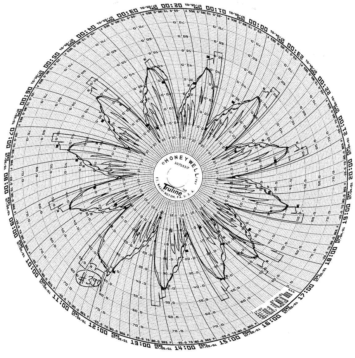
Fig. 18.1 Typical temperature history of 12 freeze-thaw cycles
