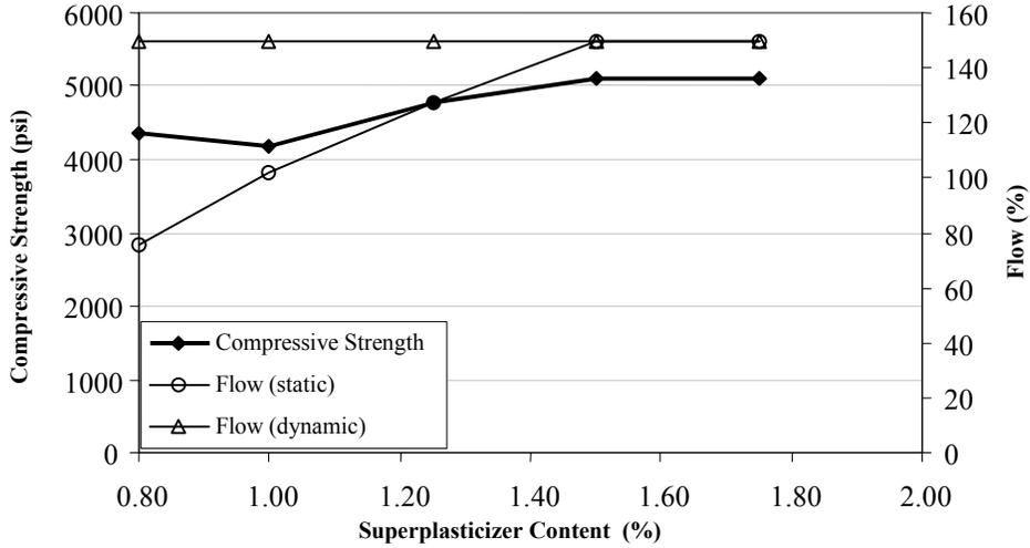
**Fig. 4.2: Test Results (Pozzolith 400N, w/c=0.47)**
