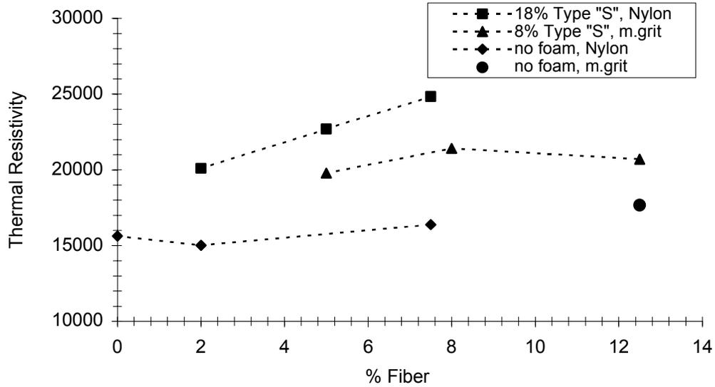
Fig. 11.4: Thermal resistivity vs. amount of fiber and foam.
