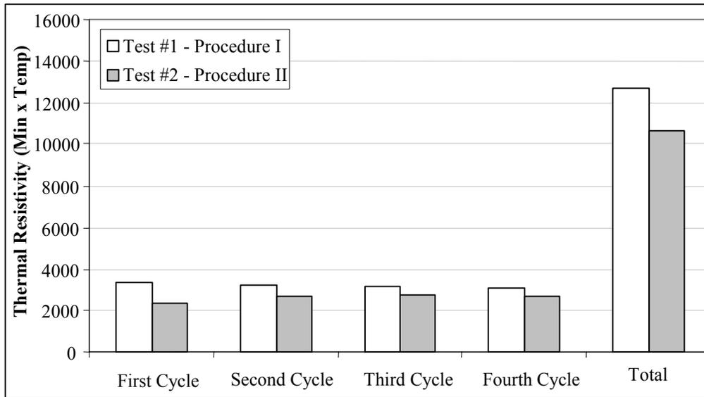
Fig. 9.7: Thermal Resistivity of Sample 72 (0% fiber) - Test Period 6 hours
