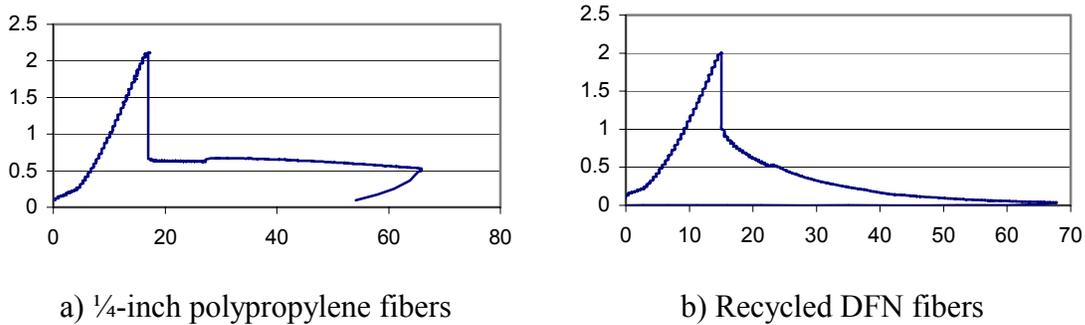
Fig. 17.3 Load (kip)-Displ. (inch/1000) Curves for Fiber-Reinforced Concrete Beams
