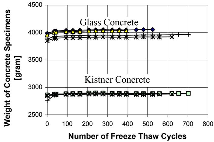
Fig. 18.4 Weight vs. number of freeze-thaw cycles.
