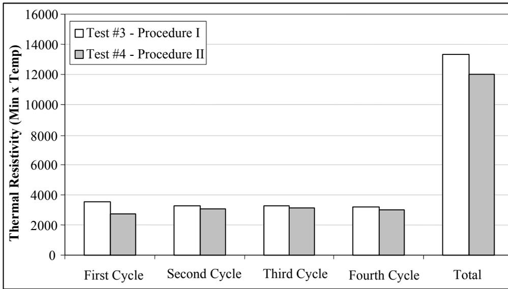
Fig. 9.8: Thermal Resistivity of Sample 77 (10% Grit fiber) - Test Period 6 hours
