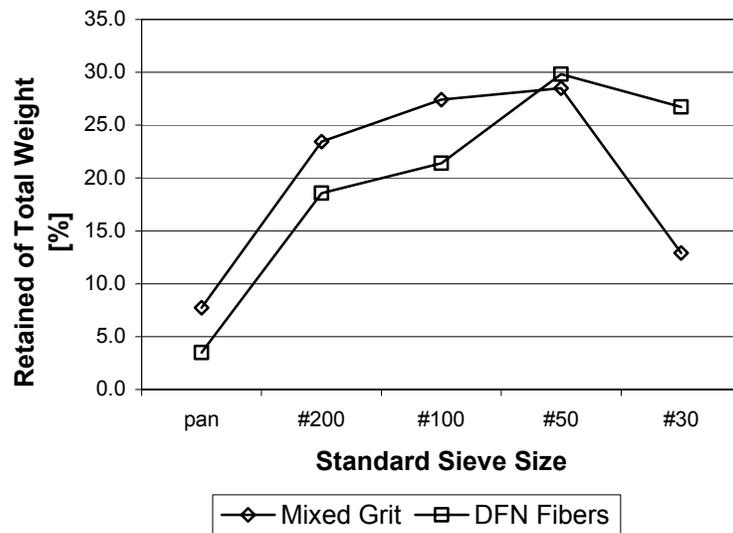
Fig. 15.2 Sieve analysis of Mixed Grit and DFN Fibers.
