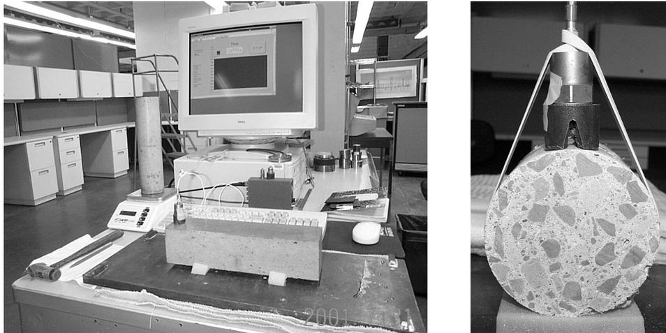
Fig. 18.2 Experimental setup to measure transverse natural frequency
