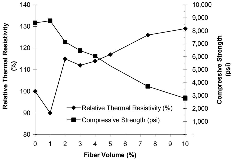
Fig. 10.2: Thermal Resistivity and Compressive Strength vs. Fiber Content – Recycled Nylon
