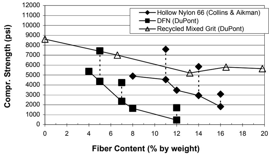
Fig. 16.3 Effect of fiber content on compressive strength (Flow > 90).
