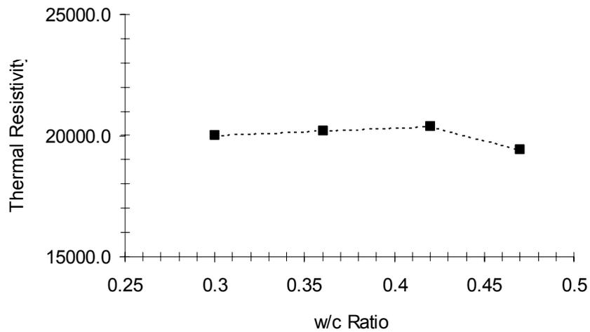
Fig. 11.6: Thermal resistivity vs. w/c ratio (18% of foaming agent type "N", 2% nylon fiber).
