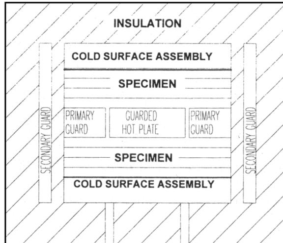
Fig. 17.1 General Arrangement of the Mechanical Components of the Guarded-Hot-Plate Apparatus
