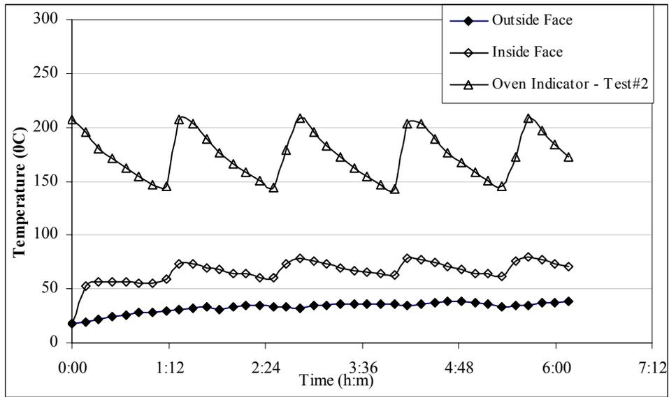
Fig. 9.4: Temperature Histories, Test #2 (Sample 72 - 0% fiber) – Procedure II
