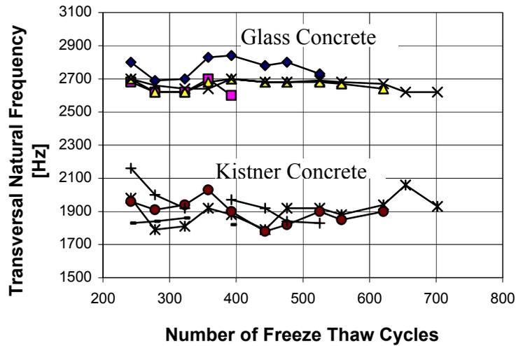
Fig. 18.5 Transverse natural frequency vs. number of freeze-thaw cycles.
