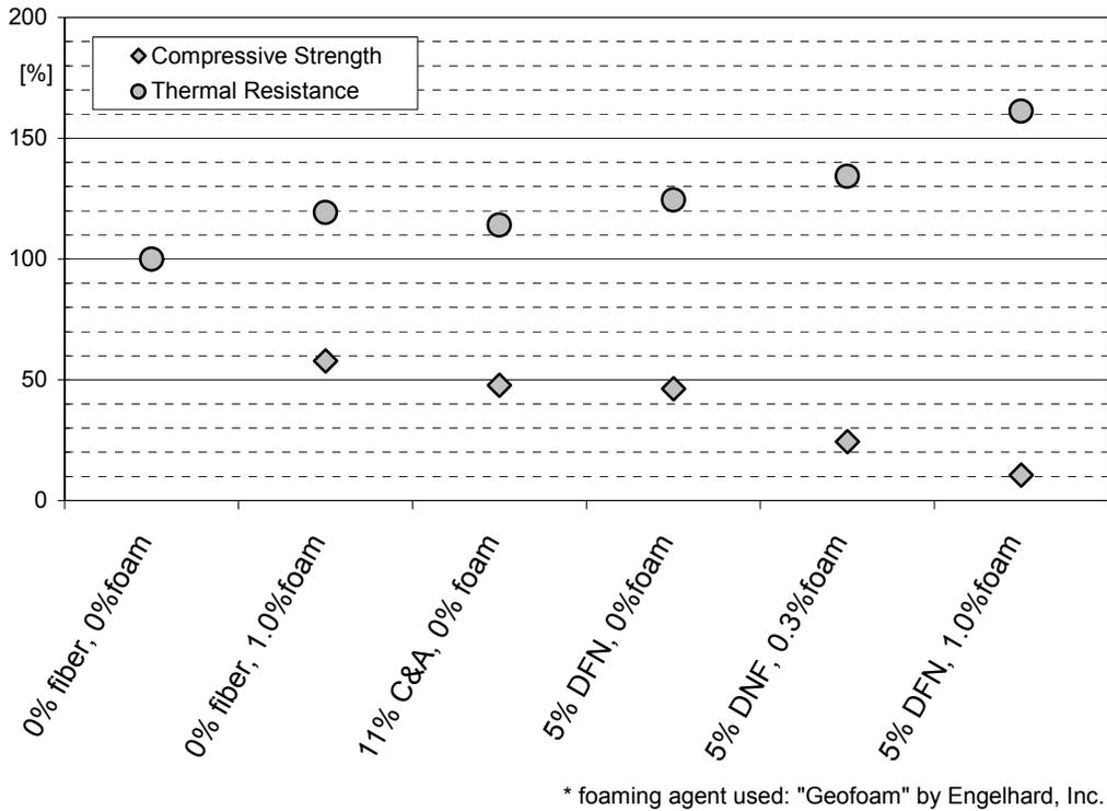
Fig. 16.5: Thermal performance and 7-day compressive strength of samples containing DFN fibers and/or foaming agent.
