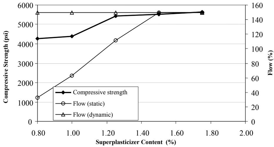
**Fig. 6.2: Test Results (Borem 900, w/c=0.47)**
