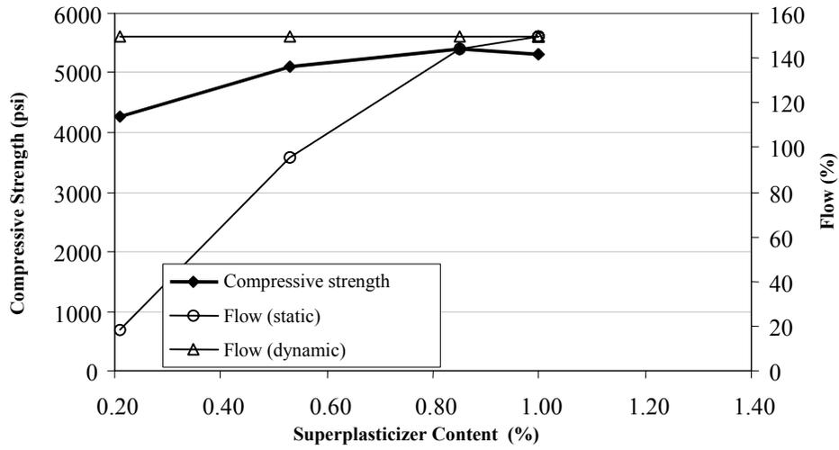
**Fig. 5.2: Test Results (Proprietary Admixture, w/c=0.47)**
