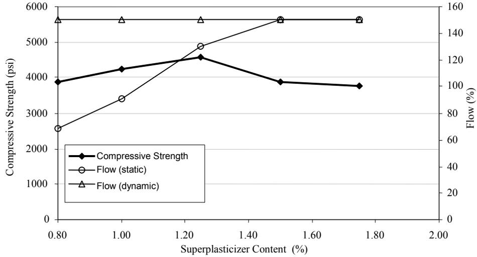
**Fig. 3.2: Test Results (Reobuild 1000, w/c=0.47)**
