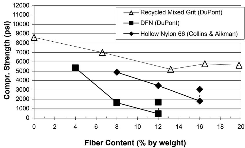
Fig. 16.2 Effect of fiber content on compressive strength (Flow > 90)
