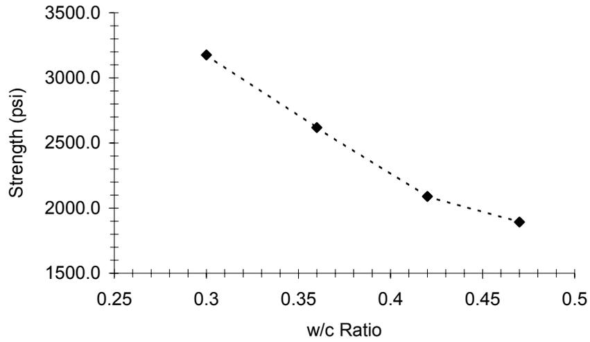
Fig. 11.3: Strength vs. w/c ratio (18% of foaming agent type "N", 2% nylon fiber).
