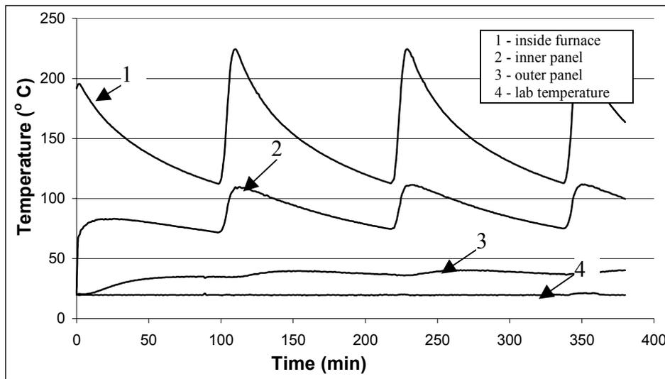
Fig. 9.3: Temperature Histories, Test#1 (Sample 72 - 0% fiber) – Procedure I
