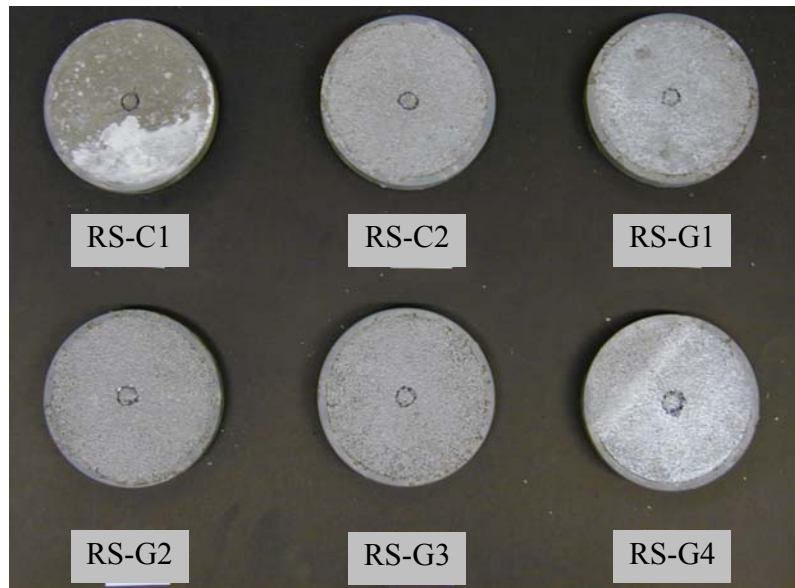
Fig.7 Typical cracking patterns of slabs after punching shear (top face) (For description of specimen IDs refer to table 2.)
