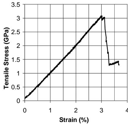
b) Stress-Strain Behavior of 8 Aramid Rovings
