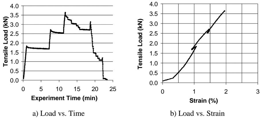
Figure 4. Response of Aramid Textile Fabric
