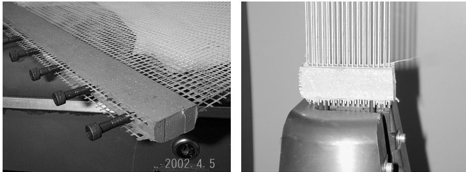
Figure 3. Epoxy Anchorage for Aramid Textile Fabric
