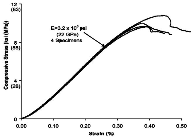
Figure 5. Glass Concrete Stress-Strain Curve
