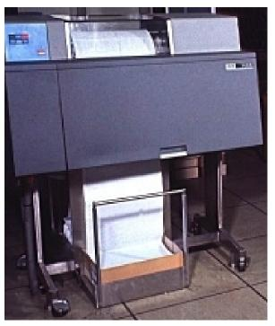
Figure 7 IBM 1403 Chain Printer
