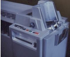
Figure 8 Punched Card Sorter. The knob in the center of the right photograph is the dial that selects a specific column to be sorted.
