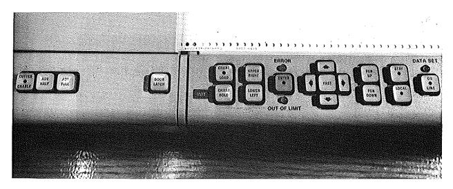
Photograph 4-4: Hewlett-Packard 7221S Front Control Panel
