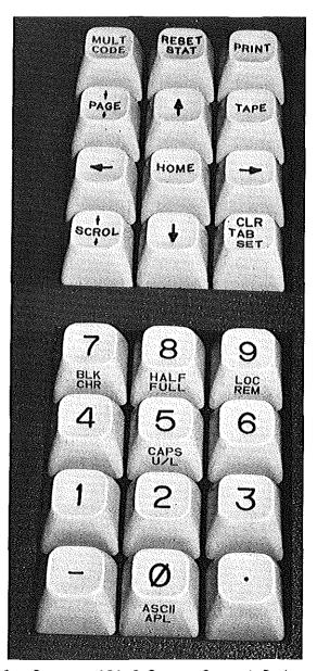
Photograph 2-3: Concept APL-8 Cursor Control Pad and Numeric Pad
