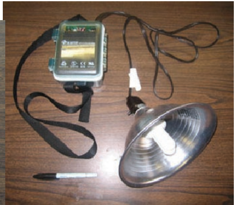
The final product designed by Columbia students: a battery with shoulder strap is attached to a lamp and reflector.
