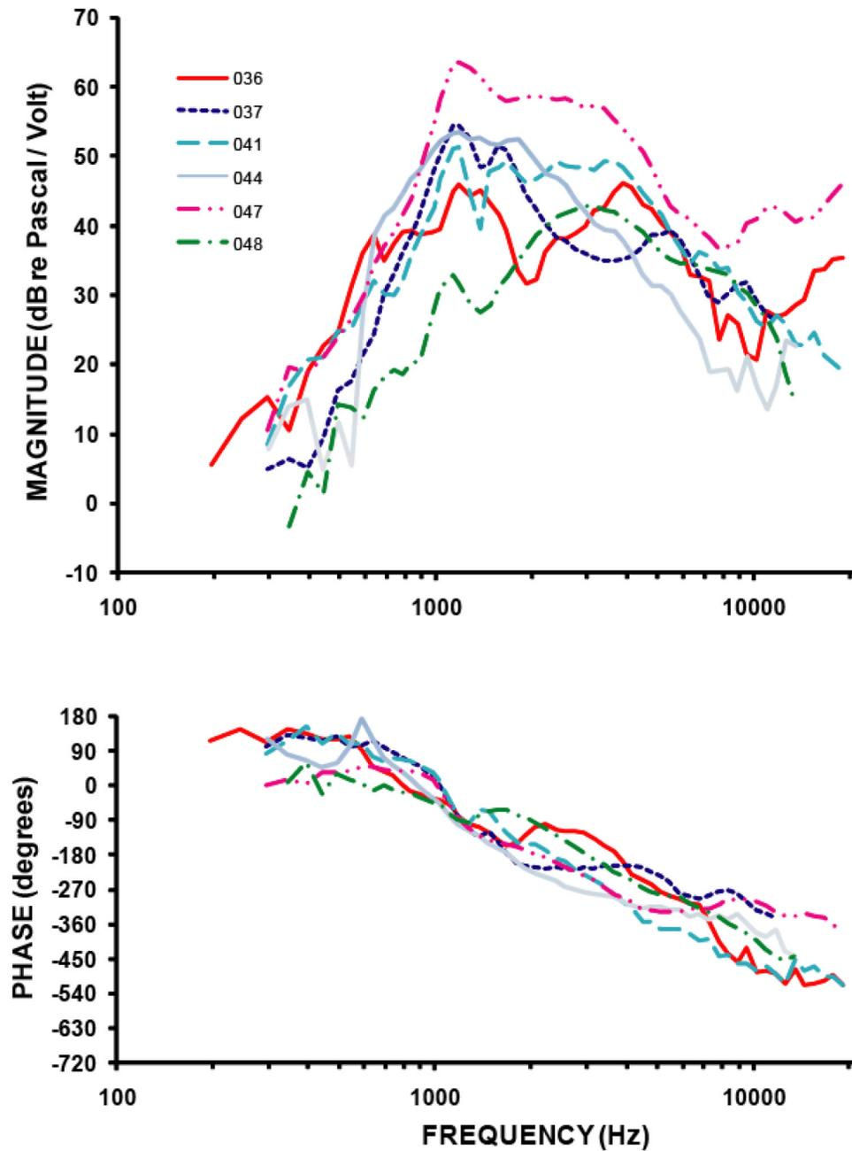
**Figure 3.** Differential pressure normalized to FMT input voltage ( $(P_{ST}-P_{SV})/V_{FMT}$ ) (the pressures that are normalized to the input voltage are subtracted in the complex domain). Each curve represents data from a different temporal bone.
