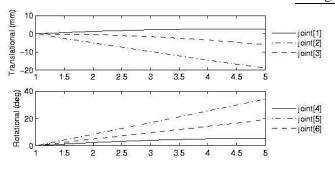
Fig. 8. Joint motions for test trajectory when using a rigid tool
