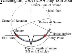
Fig. 10. Ideal path of needle tip for minimal tissue tear is a circle with the same radius as the suture needle and centered at needle center
