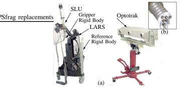
Fig. 9. Experimental setup showing (a) the LARS, the SLU Unit and the Optotrak and (b) a close-up of the SLU and gripper rigid body
