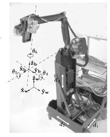
Fig. 3. The LARS robot and its kinematics
