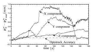
Fig. 12. X, Y, and Z components of  $\mathbf{p}_g^w - \mathbf{p}_g^w$  measured by Optotrak 3020 from Northern Digital Inc.(Accuracy 0.1mm, 1 deg), where  $\mathbf{p}_g^w$  is position of the gripper frame in world coordinates at any given instant, and  $\mathbf{p}_g^w$  start is the position of the gripper frame at the beginning of suture biting motion.
