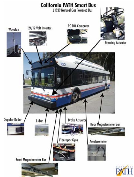
Figure 11. Hardware Setup on 40ft New Flyer Bus.
