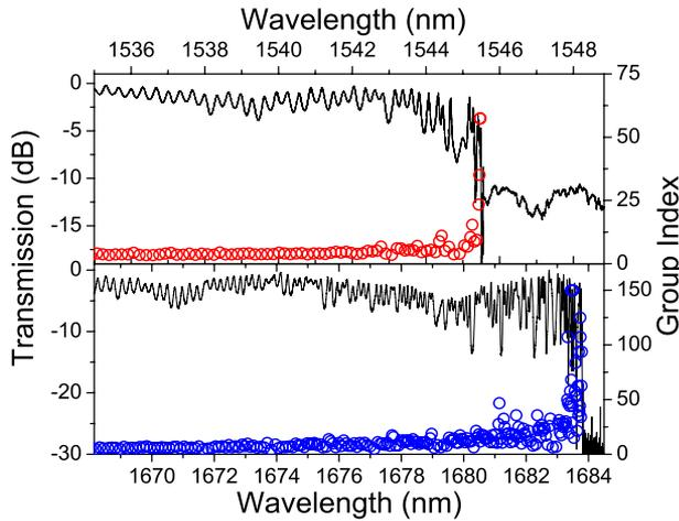
FIG. 2. (Color online) High resolution ( $\Delta\lambda=1$  pm) tunable laser transmission measurements (solid lines) and derived group index (open circles). (Top) TM polarization. (Bottom) TE polarization.
