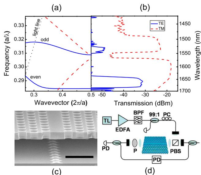
FIG. 1. (Color online) (a) Calculated projected band structure for the W1 PhCWG. (b) Measured transmission of fabricated waveguide. (c) Scanning electron microscope image of PhCWG (scale bar:  $1 \mu\text{m}$ ). (d) Experimental setup: TL, tunable laser; EDFA, erbium fiber doped amplifier; BPF, band pass filter; PC, polarization controller; P, polarizer; PBS, polarized beam splitter, and PD, photodetector.
