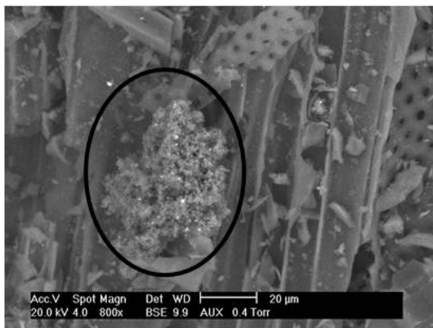
Figure 4.4: Char sample H_2O-550-30 after being used to catalyze propane decomposition. Iron cluster with carbon deposition, showing that iron is potentially a catalytic site.
