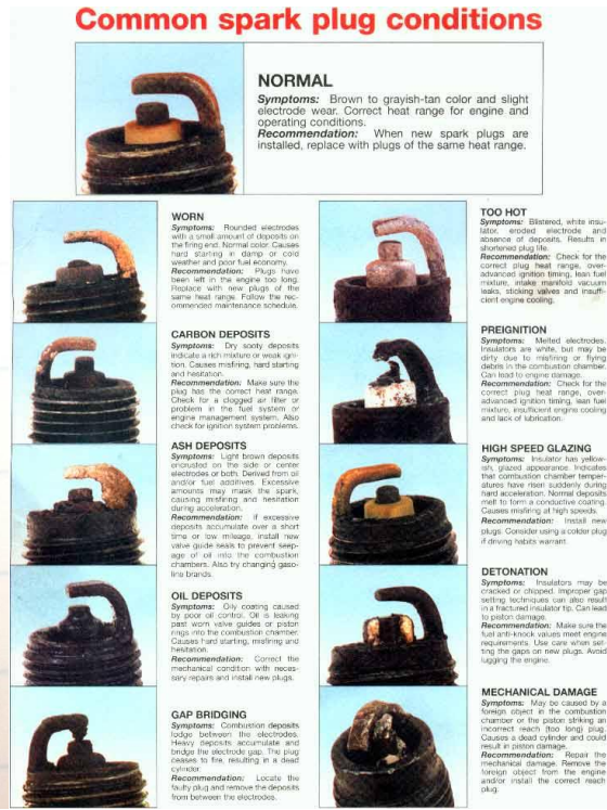
Figure 21 Spark Plug conditions and damages
