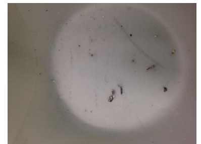
Figure 25. Deposits, founded on the valve stem neck
