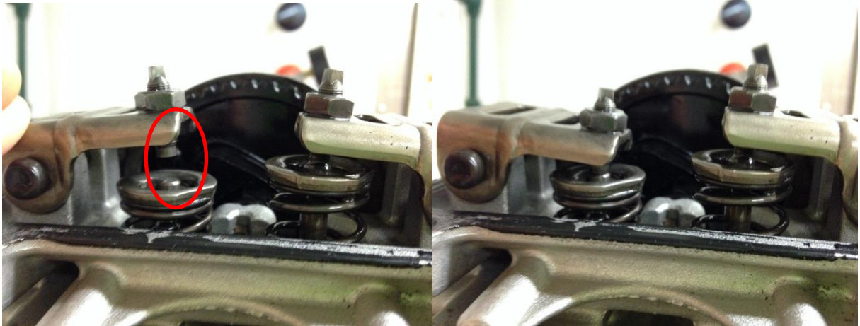
Figure 24. Cam shaft inlet and outlet at 1 and 3 stroke position
