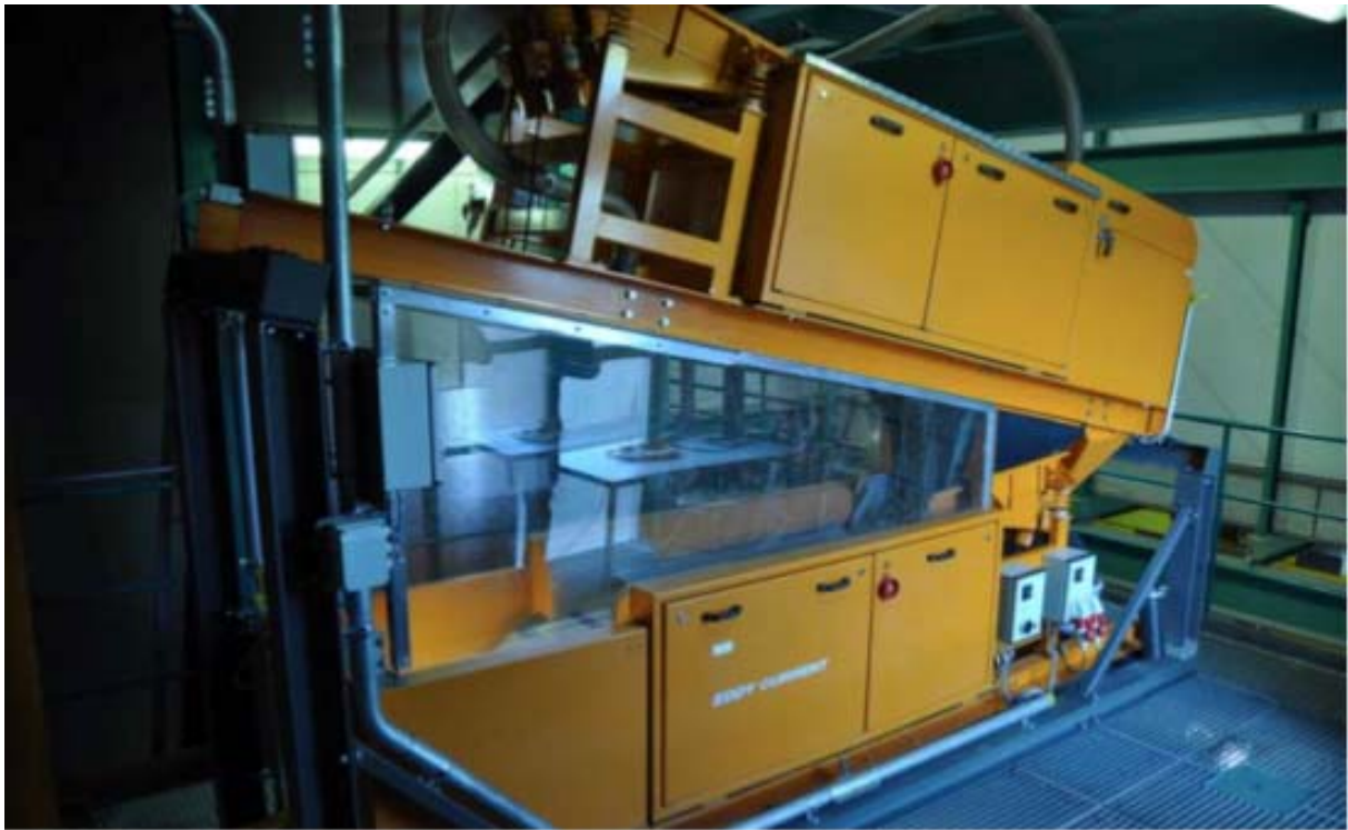
Figure 10. Eddy current separator at KEZO incinerator Zurich
