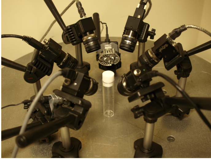
FIG. 2.1. Experimental setup of six cameras on the circular rig. Flies are placed in the vial in the center.
