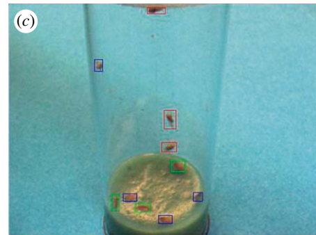
Figure 8. (a–c) Detection of fly silhouettes in two-dimensional camera images. This bounding box representation around the detected fly silhouettes shows the accuracy of the silhouette detection algorithm in distinguishing between flies when they are clumped together, as shown in (a).
