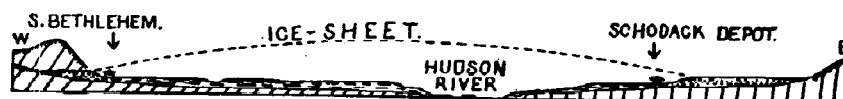
Fig. 15 Cross-section of glacial deposit in Hudson valley from Schodack Depot to South Bethlehem, showing glacial terraces where the Moordener kill and Oniskethau creek mouthed on the ice border. The rock terrace is covered by clays of later deposition.
