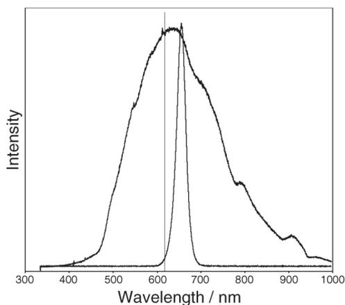
Figure 2. Comparison of spectral outputs of red traffic lights. The narrow peak with  $\lambda_{\text{max}}$  at  $\sim 640$  nm is the spectrum of the red LED traffic light. The broader spectrum is the output of an unfiltered incandescent bulb used in a traditional traffic light. When this bulb is covered with a red plastic lens, wavelengths exceeding  $\sim 600$  nm (vertical line in the figure) are transmitted, accounting for the red color.
