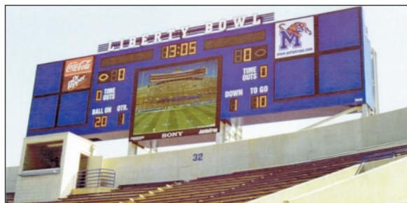
Figure 5. Giant outdoor LED displays like this Sony JumboTron in the center of the Liberty Bowl Stadium scoreboard in Memphis, TN, are being used to show live video and instant replays.
