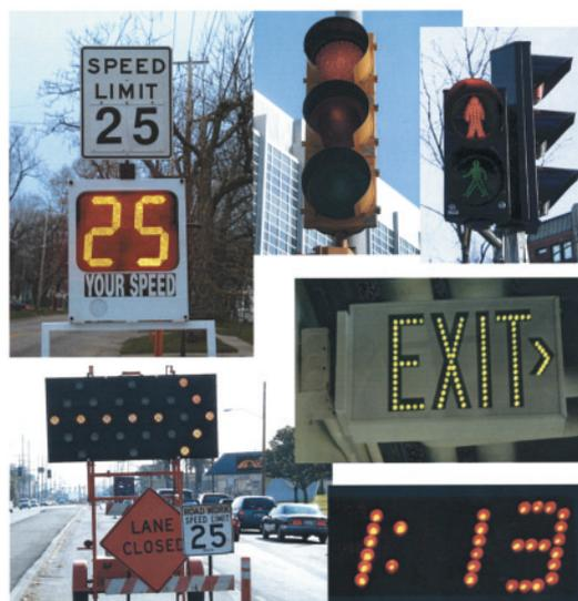
Figure 4. LEDs are being used for a variety of monochromatic applications, such as (clockwise from upper left) speed indicators, traffic and pedestrian signals, exit signs, large digital clocks, and construction arrows.
