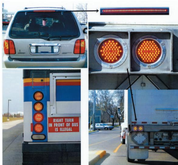
Figure 3. Illustrations of LED vehicle applications. Clockwise from middle right: close-up view of truck brake lights, and their position on the vehicle; bus brake lights and turn signals; automotive center high mount stop lamp (CHMSL) and closer view.
