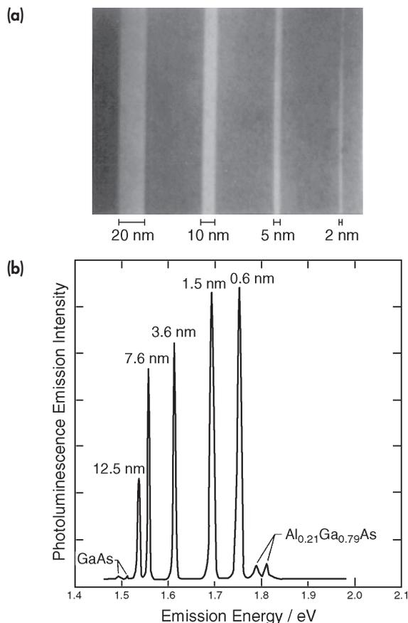
Figure 8. (a) Chemical composition can be controlled at the nanoscale. This scanning electron microscope (SEM) image shows various thicknesses of GaAs layers sandwiched between thicker (50-nm)  $\text{Al}_{0.3}\text{Ga}_{0.7}\text{As}$  layers, forming so-called quantum wells. (b) Emission from a set of quantum wells like those shown in (a), illustrating that emission energy increases as thickness, labeled on the spectrum, decreases.
