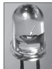
Close-up of an LED assembly. The LED itself is the tiny chip that is indicated by the arrow.
