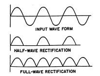
Recently some X-ray manufacturers have used **amplifiers** to increase the number of cycles and are claiming that they are obtaining a **continuous direct current r**esulting in a current that has higher energy at the same voltage.
