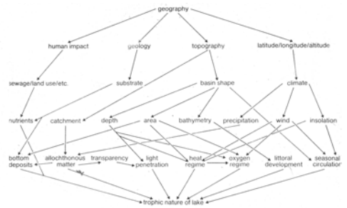
Interrelationships of the main factors affecting the trophic status of a lake:
