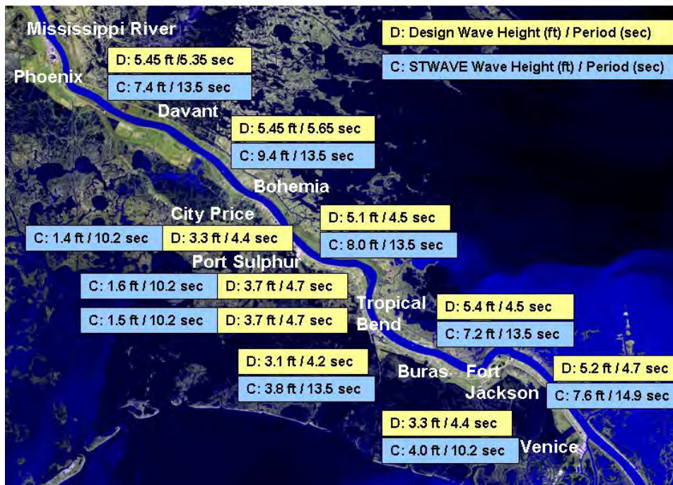
Figure V-44. Wave maxima along hurricane protection levees in Plaquemines Parish
