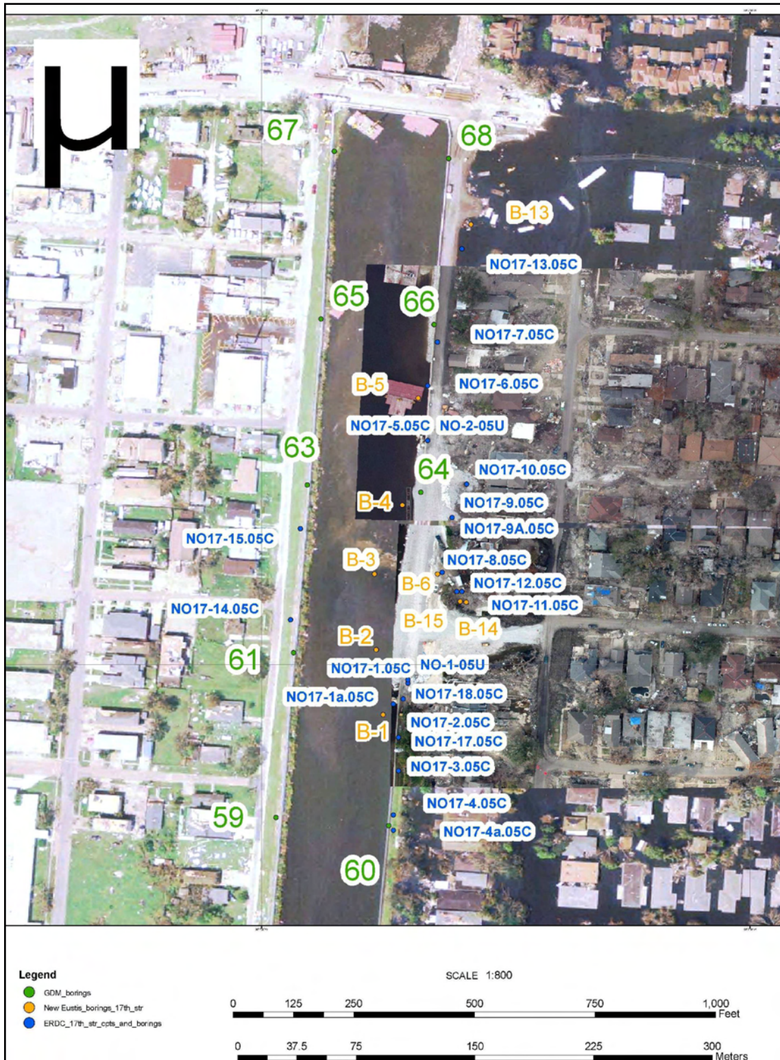
Figure VI-15. Boring and CPT Location Map
