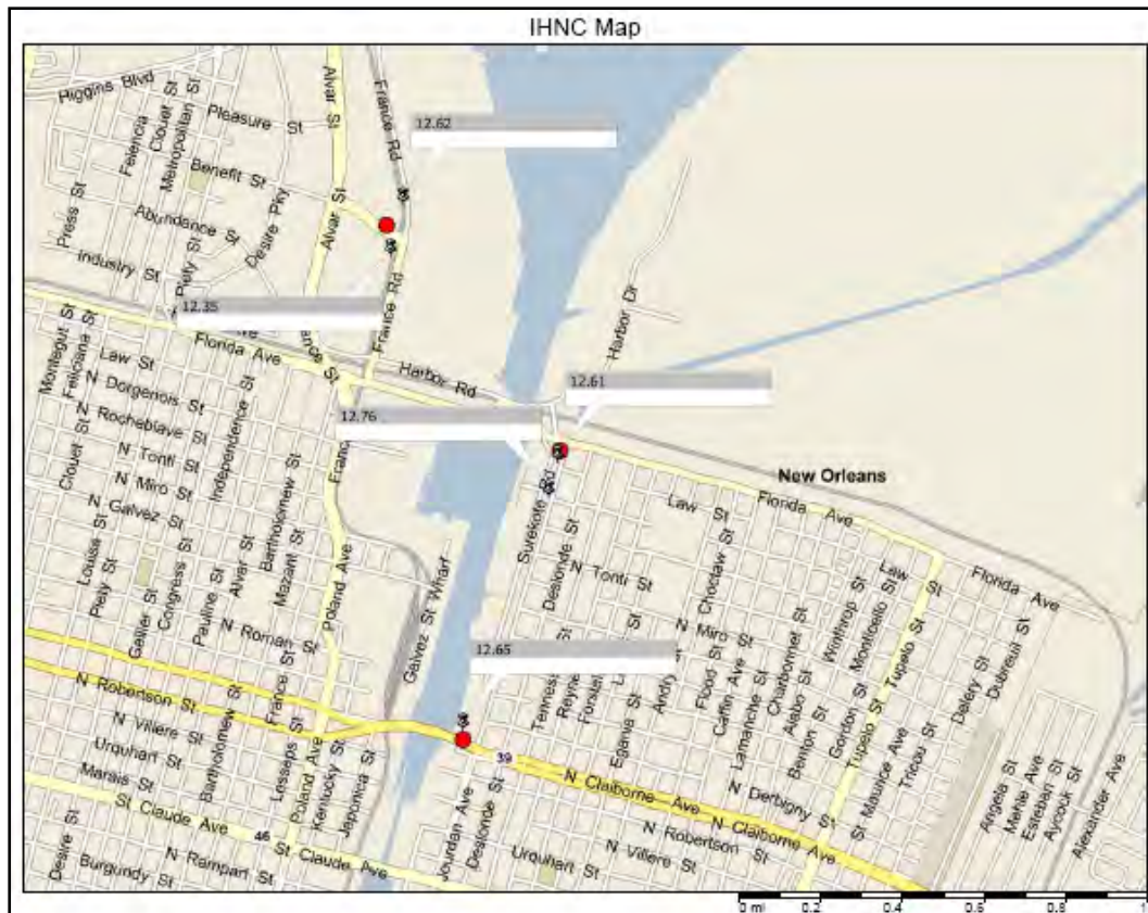
Figure III-13. Selected Post-Katrina Elevations on IHNC Floodwalls
