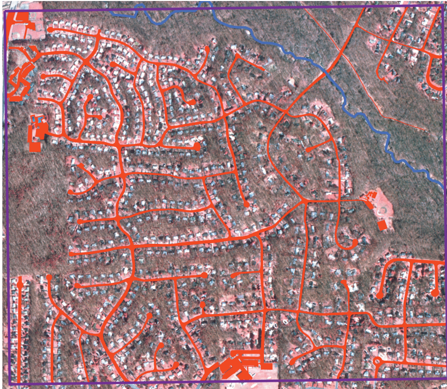
Figure 3. Direct impervious surface compilation method. Delineated roads, parking lots and commercial/institutional rooftop areas are mapped in red. The Accotink Creek is mapped in blue.
