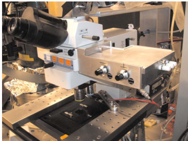
FIG. 5. (Color online) Light-tight attachment for fluorescent-signal detection using a dichroic mirror and PMTs.
