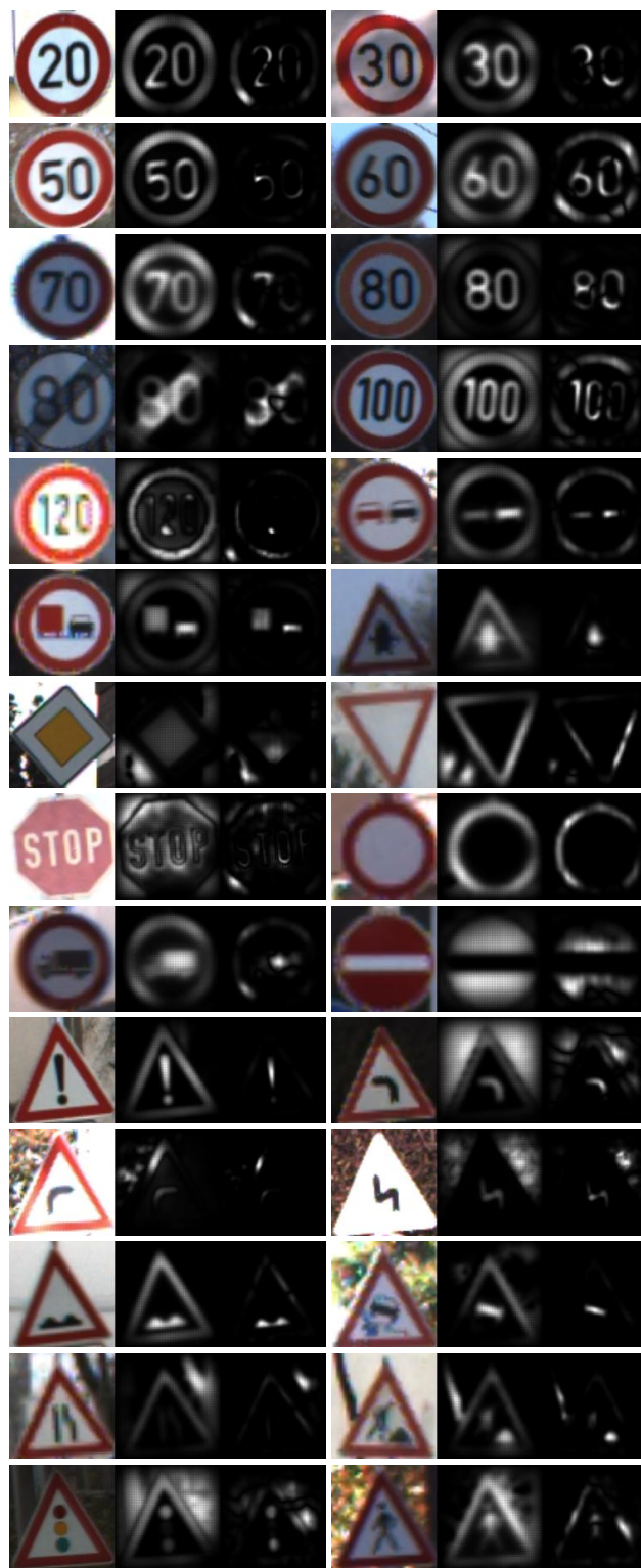
Figure 20. Sets of input images with visualization masks arranged in two columns. Each set consist of an input image (left), a visualization mask generated by VisualBackProp (center), and a visualization mask generated by LRP (right).
