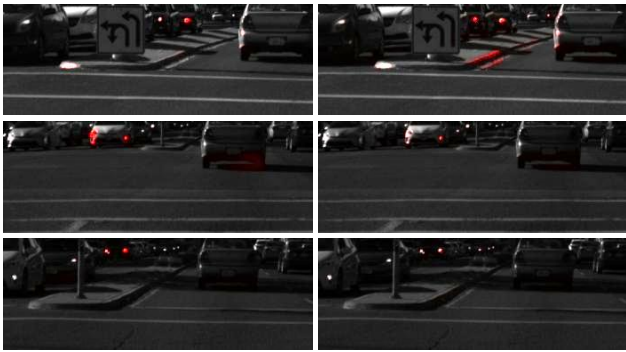
Figure 17. Network NetHVF . Left: VisualBackProp, right: LRP. Input test image with the mask overlaid in red. The errors are (from the top): -7.72 , -0.72 , and -3.17 degrees of SWA.
