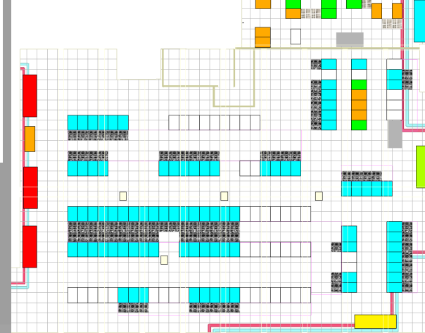
Iteration #3 – CRAC Cooling % / ASHRAE Cabinet Compliance
