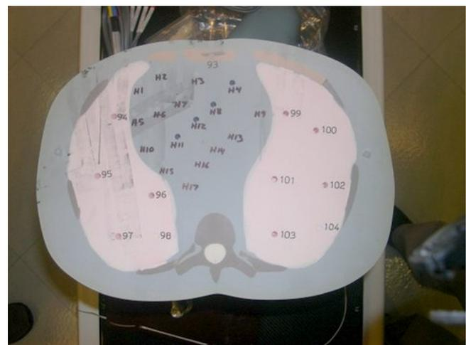
FIG. 2. Picture of one slice of the phantom. Marks indicate MOSFET positions.
