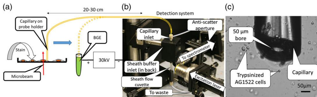
Figure 2. (a) Layout of the proposed microbeam-coupled CE-LIF system. After loading a cell into the capillary, the capillary tip is transferred to a grounded vial of BGE and negative high voltage is applied at the outlet of the sheath flow cuvette. (b) Prototype sheath flow LIF system constructed at RARAF. (c) Loading a single whole cell out of a cell suspension into a capillary at UIUC.
