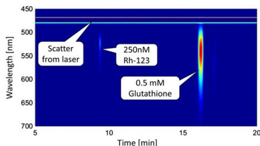
Figure 3. Wavelength-resolved electropherogram of 10 nl of a mixture of 0.5 mM glutathione derivatized with NDA and 250 nM of Rh-123. The Rh-123 signal-to-noise ratio is ~1500.
