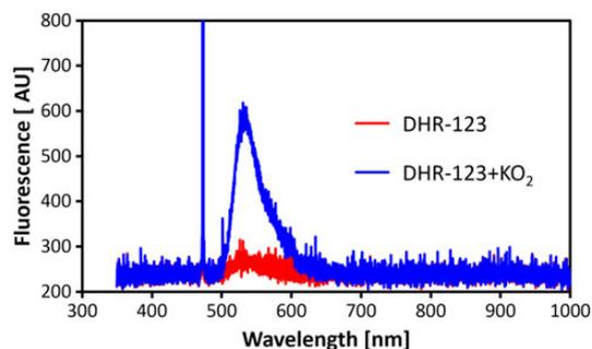
Figure 1. Fluorescence spectra measured using the RARAF breadboard LIF system of DHR-123 before (grey) and after (black) addition of  $KO_2$ , a superoxide generator. The spike at 473 nm is scattered light from the excitation laser.
