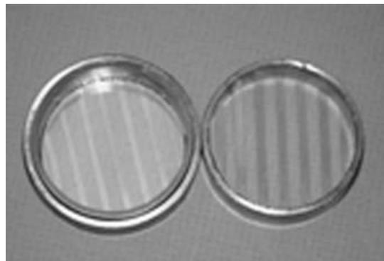
Figure 1. Double-ring apparatus used. The inner ring (internal diameter 35 mm) with 38- $\mu$ m mylar strips (width 2 mm) is shown on the right with the complete double-ring apparatus on the left (outer ring diameter is 38 mm).
