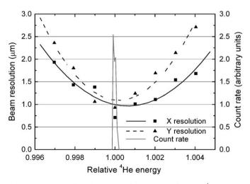
**Fig. 8.** Measurement of the degradation of the resolution for 6 MeV <sup>4</sup>He ions as a function of the relative ion beam energy. The curved lines are least squares fits to the measured points using a second-order polynomial. Also shown is the energy acceptance of our beam line optics (solid gray line).
