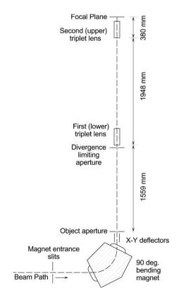
Fig. 6. Diagram of the charged particle beam optics system.
