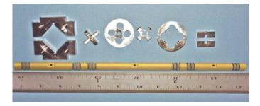
**Fig. 3.** Photograph of the electrostatic lens components (L–R): V-blocks used to clamp the lens rods; assembled cross spacer; field shaping disc; inner (cross) and outer (ring) parts of the field shaping disc; and two halves of a cross spacer. Below these components is one of the ceramic rods for a quadrupole triplet.
