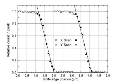
**Fig. 7.** Typical orthogonal knife-edge scans across a focused 6.0 MeV <sup>4</sup>He beam. The lines are linear least-squares fits to the filled points.
