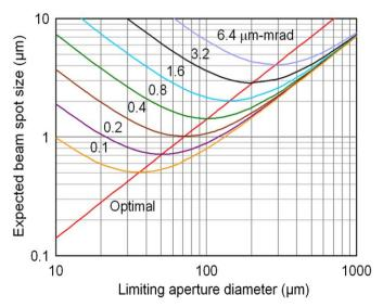
**Fig. 4.** Results of calculations of the beam spot diameter produced by the compound electrostatic quadrupole triplet as a function of the diameter of the angular divergence limiting aperture for various diameters of the object aperture. The curves are for constant emission ( $\mu$ m-mrad). The values of the limiting aperture diameter that results in the minimum beam spot diameter for given particle transmission are connected by the diagonal line.
