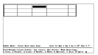
When you expand the width of cell C1, the width of cell D1 (the widest cell to the right of C1) decreases.
