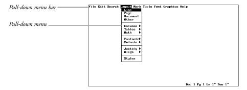
The pull-down menus can be accessed with the keyboard. A list of the items on the pull-down menus can be found in Appendix N: Pull-Down Menus.
