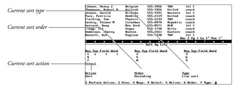
All of the current sort criteria are displayed. At the bottom of the screen is a menu of options which you can use to change the sort (and select) criteria.
