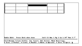
When the Table Edit menu is displayed, you can also increase and decrease column widths in one-character increments by moving the cursor to a column and pressing Word Right to increase width and Word Left to decrease width.
