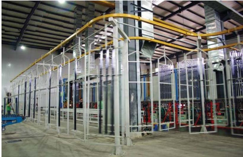
**Plate 14. Fully automatic facility for manufacturing of evacuated tubes.** Top, the automatic evacuating machine. Bottom, the automatic conveying line. That facility alone produces 20 millions of evacuated tubes each year, with rated power more than that of Europe and U.S. combined. Courtesy of Himin Solar Energy Group, Dezhou, China.
