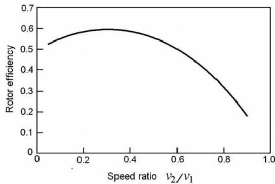
**Fig. 1.11. Efficiency of wind turbine.** The efficiency of wind turbine as a function of the ratio of wind speed after the rotor and the wind speed before the rotor. As shown the maximum efficiency is  $16/27$ , which occurs at a ratio of  $1/3$ .
