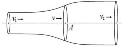
**Fig. 1.10. Derivation of the Betz theorem of wind turbine.** The wind velocity before the turbine rotor is  $v_1$ , and the wind velocity after the turbine rotor is  $v_2$ . The velocity at the rotor is the average velocity, and the power generated by the rotor is related to the difference in kinetic energy.
