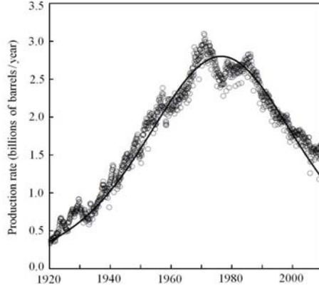
**Fig. 1.6. Rate of production of crude oil in the US.** Circles: actual production rate of crude oil on the US. Source of data: EIA (The United States Energy Information Administration). Solid curve: the Hubbert function, using a least squares fit to the actual data. The sudden increase of production at 1977 and the second peak at 1989 are due to the starting of oil production in Alaska, see Fig. 1.7.
