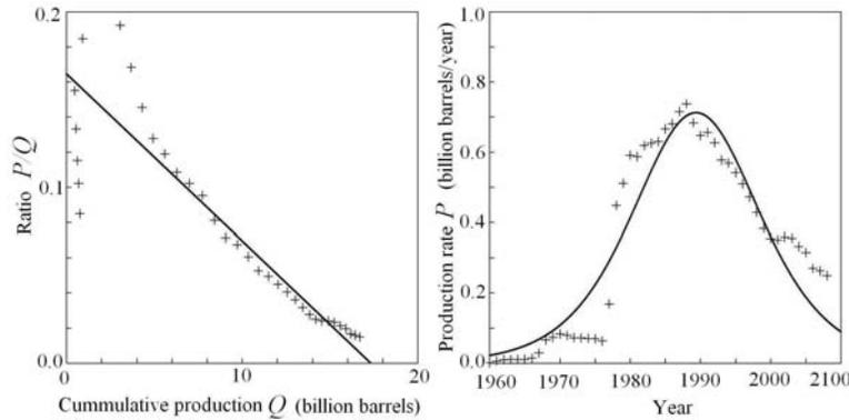
**Fig. 1.7. Production of crude oil in Alaska.** (a) The ratio of  $P/Q$  versus  $Q$  for Alaska. Source of data: EIA. Except the earlier years, the ratio shows a rather accurate linear dependence on  $Q$ . From the plot one finds  $Q_0 = 17.3$  billion barrels,  $a = 0.1646$ , and  $t_m = 1989.38$ . (b) A Hubbert curve is constructed. As shown, except in the early years, the production data follows the Hubbert curve rather accurately.
