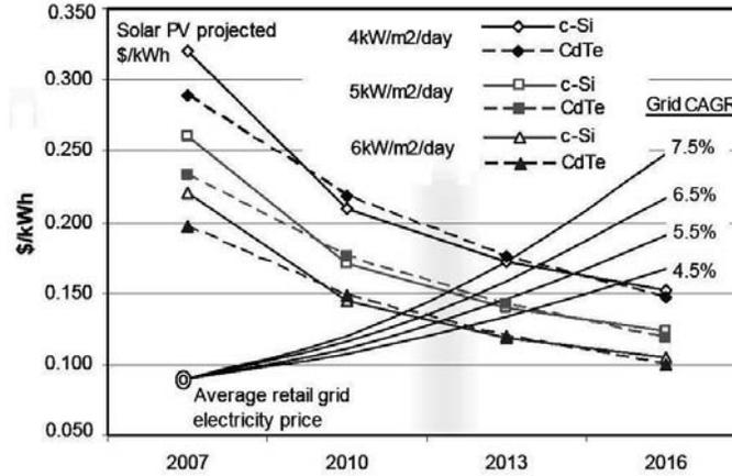
**Fig. 1.37. Prediction of grid parity.** According to the forecast of Deutch Bank, two most promising solar cell technology, crystalline silicon solar cells and CdTe thin film solar cells, will arrive at grid parity around year 2013. Beyond 2013, the cost of solar electricity could be lower than that of traditional source of electricity for many places of the world. After *Solar Photovoltaic Industry, 2008 global outlook*, Deutch Bank.
