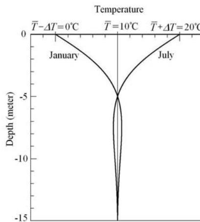
tity. In much of the temperate zone, it can be used directly for space cooling. By placing heat exchange structures underground and guide the cool air through ducts to the living space, a virtually free air conditioning system can be built. In areas with average temperature close to or slightly below  $0^{\circ}\text{C}$ , underground caves can be used as refrigerators, also virtually free of energy cost.
