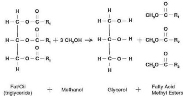
**Fig. 1.15. The production process of biodiesel.** By mixing triglyceride with alcohol, using a catalyst, the triglyceride is transesterified to form three esters and a free glycerin. The esters, or the biodiesel, has a much smaller molecule size, which provides better lubrication to the engine parts.
