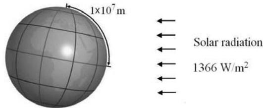
**Fig. 1.1. Annual solar energy arriving at the surface of Earth.** The average solar power on the Earth is 1 kilowatt per square meter. The length of the meridian of Earth, according to the definition of a meter, is 10,000,000 meters. The total solar energy arrive at the surface of Earth per year is 2,730,000 EJ.
