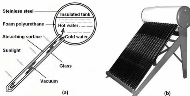
**Fig. 1.32.** The evacuated-tube solar water heater. (a) A schematic of the evacuated-tube solar water heater. Each heat collector is a double-walled glass tube. The system works automatically under the principle of natural convection. (b) A photograph of such a system.
