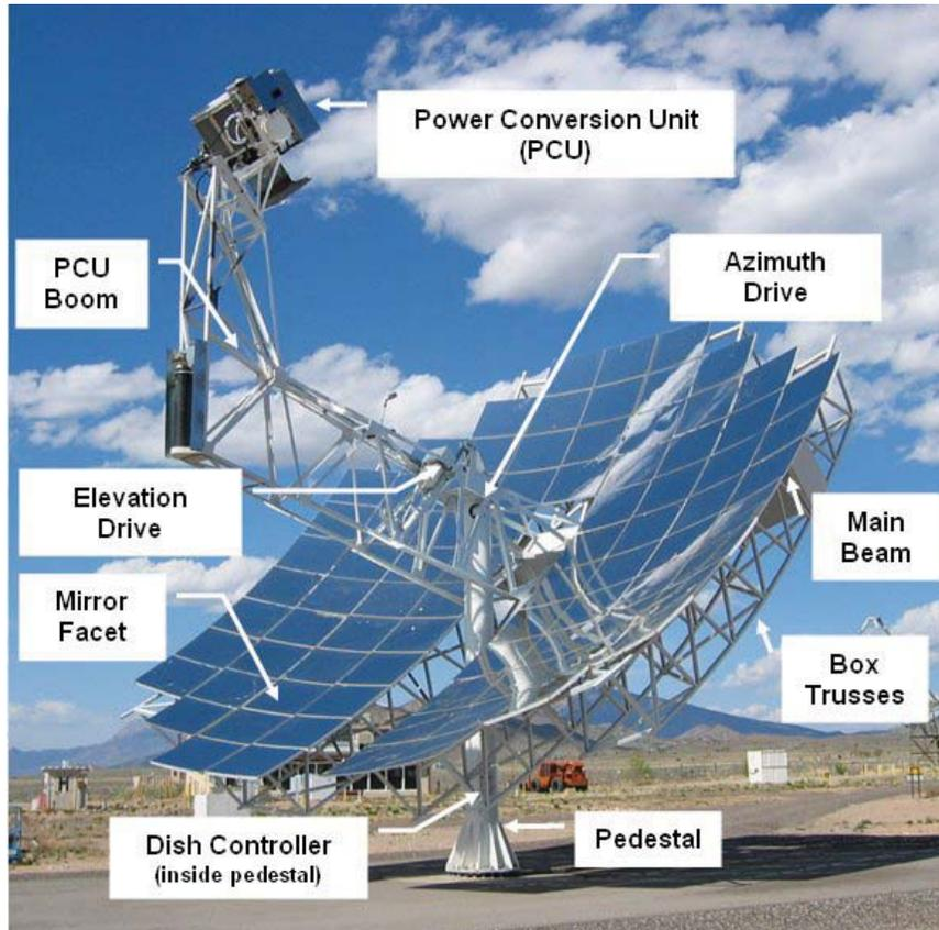
**Plate 10. Solar dish Stirling energy system.** The Stirling solar energy system developed by Sandia National Laboratories and Stirling Energy Systems (SES) in February 2008 has set a record of the highest solar-to-grid conversion efficiency of 31.25%. The solar dish generates electricity by focusing the radiation from the Sun to a receiver, which transmits the heat energy to a Stirling engine filled with hydrogen. The Stirling engine works best in a cold but sunny weather.
