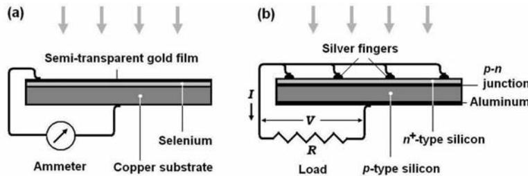
**Fig. 1.22. Selenium solar cell and silicon solar cell.** (a) Selenium photovoltaic cell was discovered in the middle of 19th century, and were used as a device for measuring light intensity for photographers. (b) Silicon photovoltaic cell was invented in Bell Labs in 1954 using the technology for silicon transistors.
