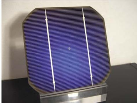
**Plate 6. Monocrystalline silicon solar cell.** The typical mono-crystalline silicon cell is cut from a cylindrical single crystal of silicon. After a *pn* junction is formed by a diffusion process, a net of interconnections, usually made of silver, is formed by screen printing process.
